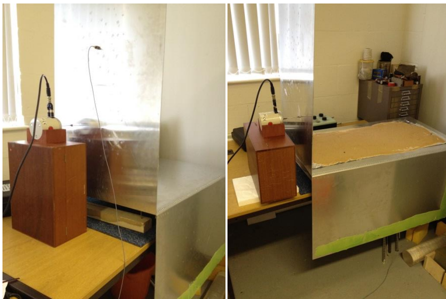
Figure 7-20 Experiment setup for energy level difference measurement
