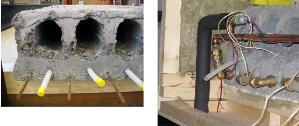
Figure 2.2 - Thermal Active Building System (TABS) [24]
