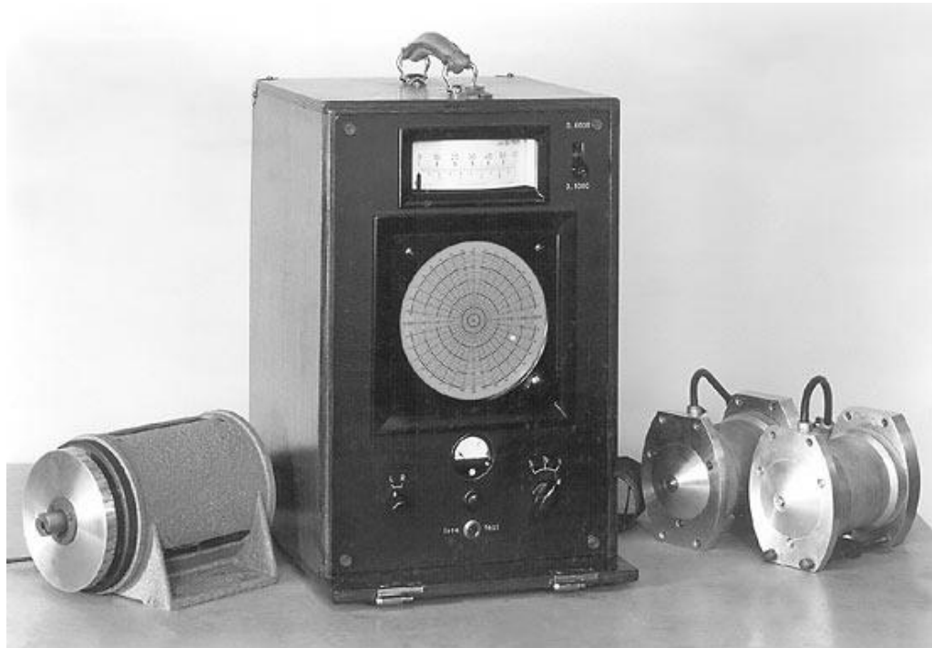
Figure 38 An illuminated-spot vectormeter within a single box allowing the user visualise the unbalance for the first time [9]
