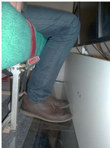
Figure 5-2 Adjustable board designed to limit the legroom of participants
