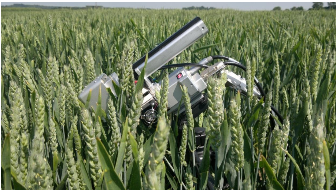
Plate 3.5 LiCor 6400-XT Photosynthesis system used for measuring leaf gas-exchange, leaf chamber clamped a wheat leaf at anthesis.
