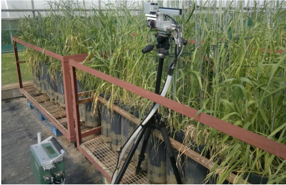
Plate 3.10 LiCor 6400-XT Photosynthesis system used for measuring leaf gas-exchange, leaf chamber clamped on a wheat leaf at anthesis.
