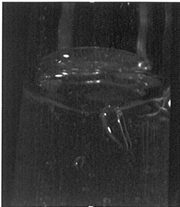
Figure 8.9: Wake of a standing bubble showing entrained gas at liquid superficial velocities 0.29m/s and gas superficial velocity of 0.02m/s with air-high viscosity oil
