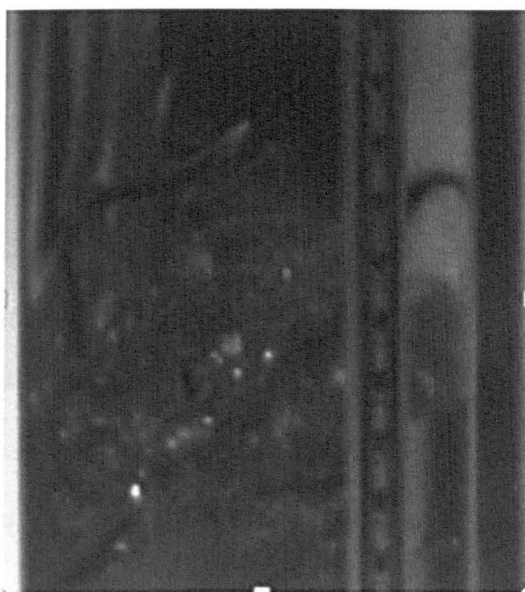
Figure 8.10: Wake of a standing bubble showing entrained gas at liquid superficial velocities 0.29m/s and gas superficial velocity of 0.02m/s with air-low viscosity oil
