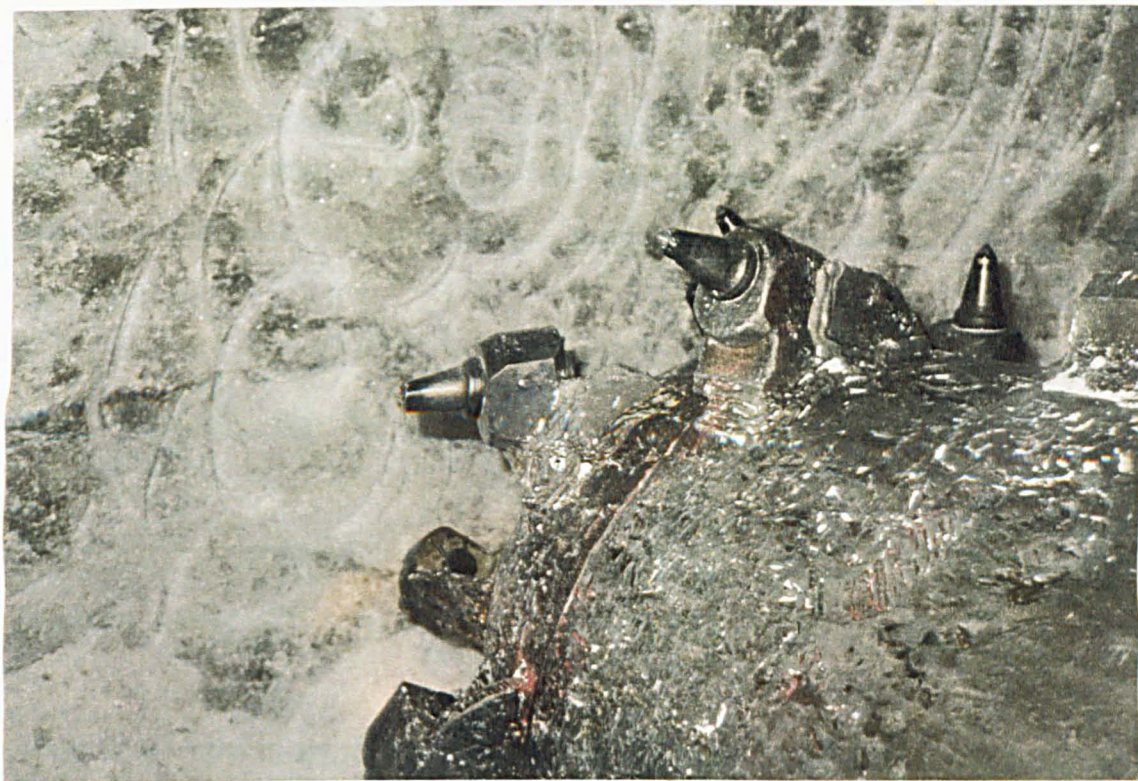
PLATE 5.1 PICK TIP FAILURE
