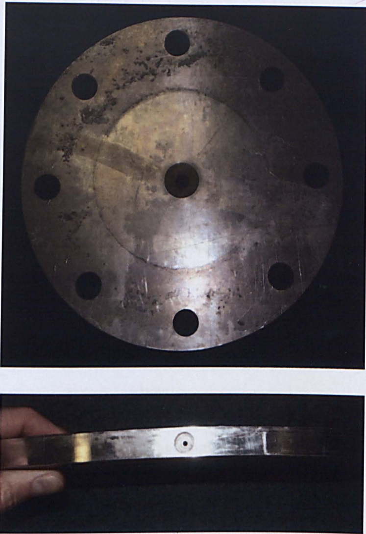
Figure 3-6: Orifice plate for creating accelerated jet of steam and injection of liquid phase
