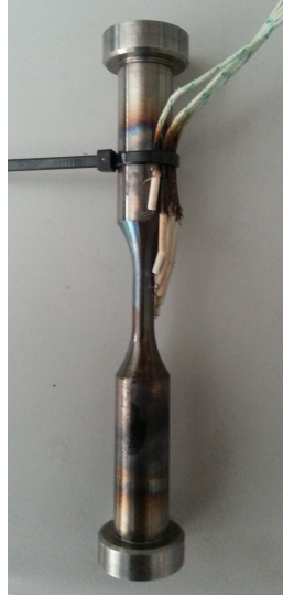
Figure 3.3: An example calibration specimen used for the design of a RF induction heating coil.
