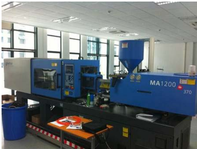
Figure 3-16 Haitian MA1200/370 injection moulding machine
