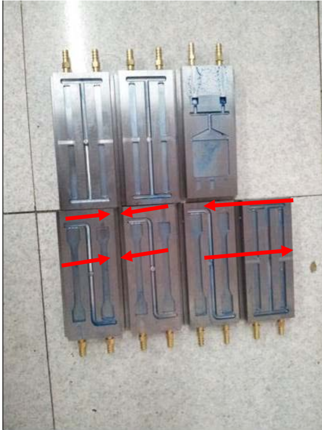
Figure 6-7 The moulds and the directions of their flow-passages as indicated by red arrows
