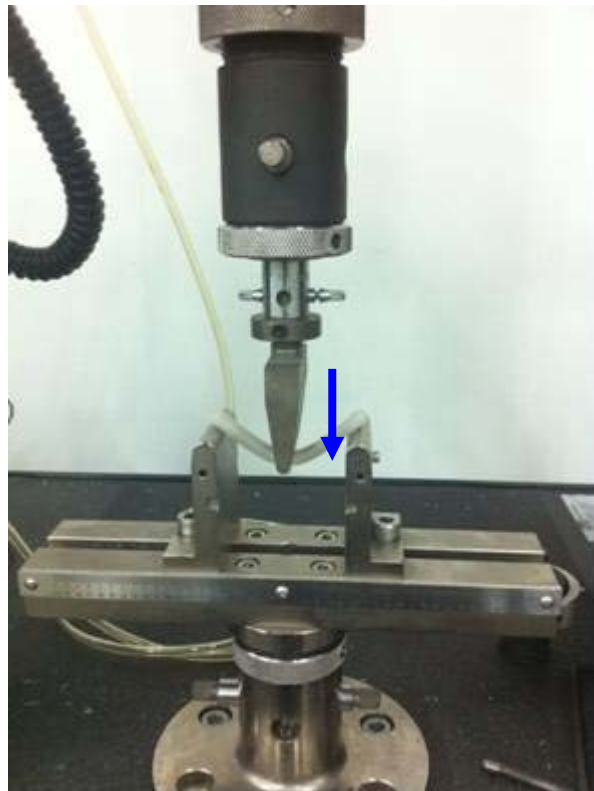
Figure 6-8 Direction of flexural testing force applied on specimens
