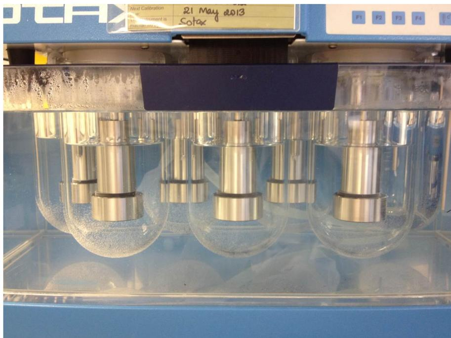
FIGURE 2.8: Rotating disk system in the dissolution equipment.
