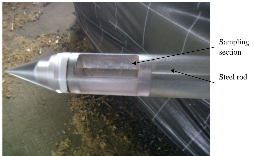
Figure 3-13. Aperture on probe and sampling section
