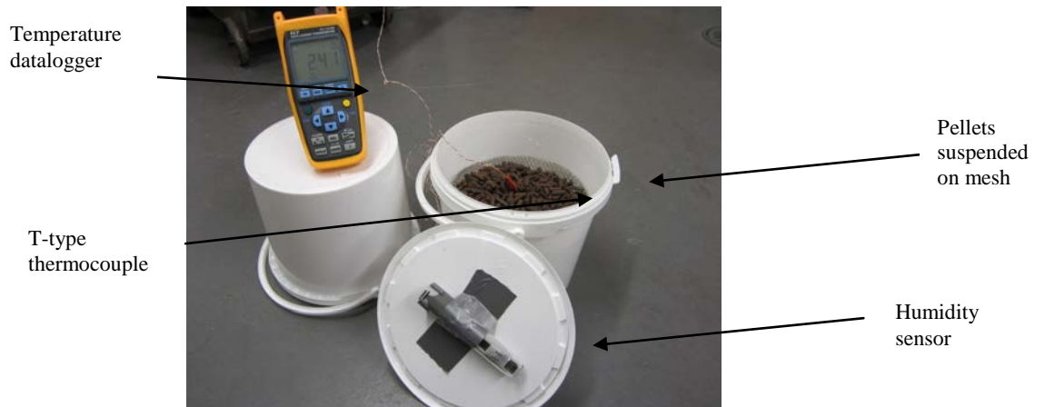
Figure 1: Instrumentation set up for enclosed high humidity trials, before sealing.
