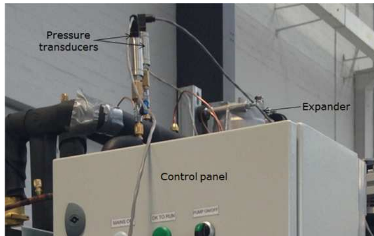
Figure 7-31: Pressure transducers installed on the ORC prototype.
