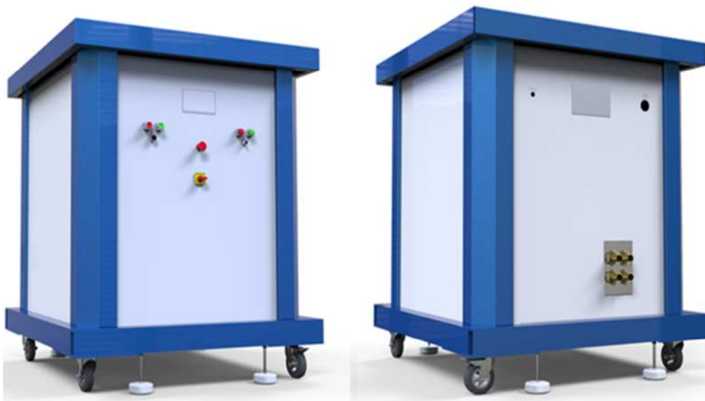
Figure 7-3: 3D illustrations of the R1233zd(E) ORC prototype system with rugged industrial casing.
