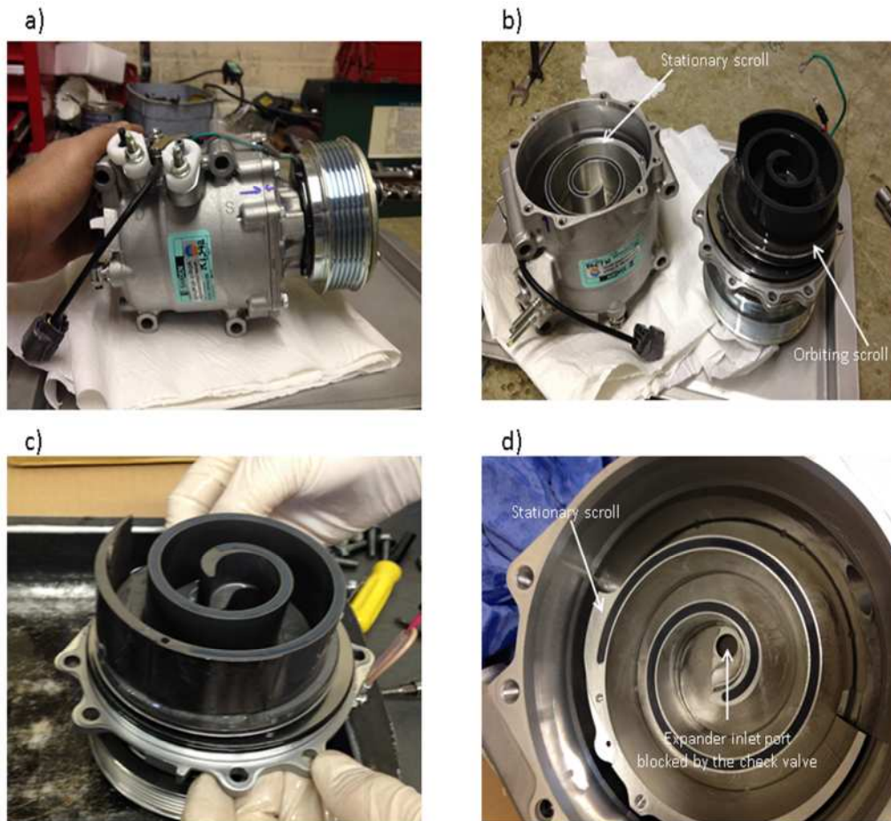
Figure 7-10: Views of scroll compressor modification procedures 1- a) side view of the TRSA09 compressor prior modification, b) the dismantled compressor showing stationary and orbiting scrolls, c) a zoomed-in view of the orbiting scroll, and d) a zoomed-in view of the stationary scroll, showing the expander mode inlet port blocked by the check valve.
