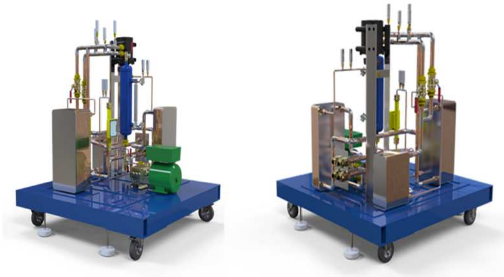
Figure 7-2: 3D illustration of the R1233zd(E) ORC prototype system.
