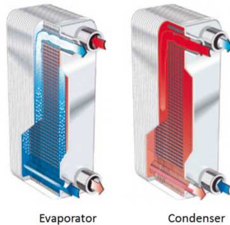
Figure 7-26: A BPHE as an evaporator and condenser in a refrigeration system. (Source: [285])
