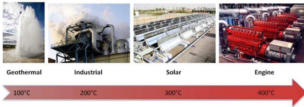
Figure 2-6: Variation of heat source temperatures in different ORC applications. (Source: [86])
