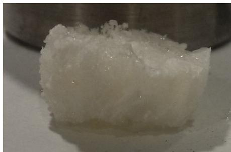
**Figure 5-8. Foamed PDLLA product directly from the autoclave**
