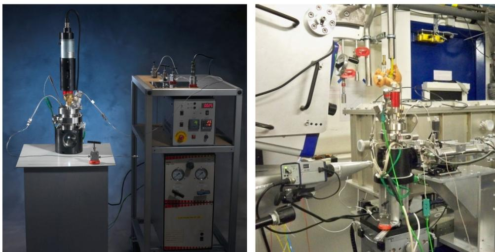
**Figure 2-12(Left) High pressure cell with pump and control box. (Right) Cell aligned in the beamline with SAXS and WAXS detectors.**
