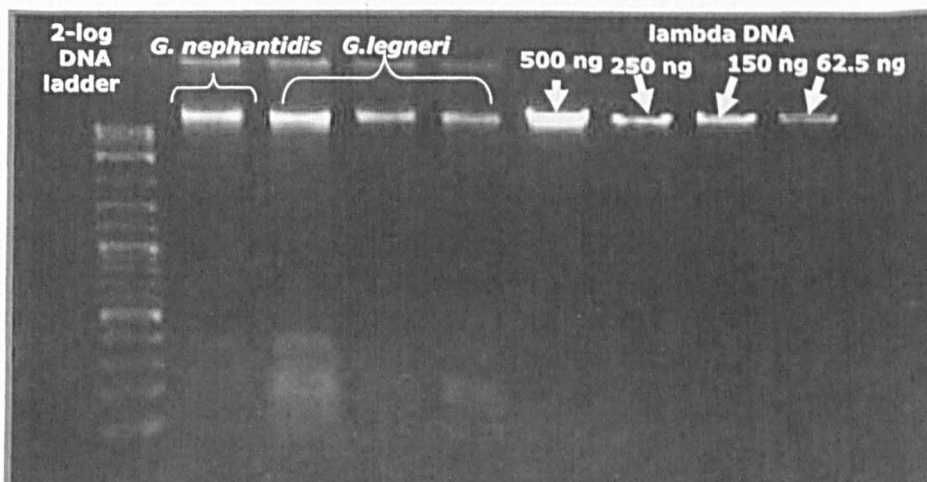
Figure 5.3 Quality and quantity test for Goniozus DNA templates
