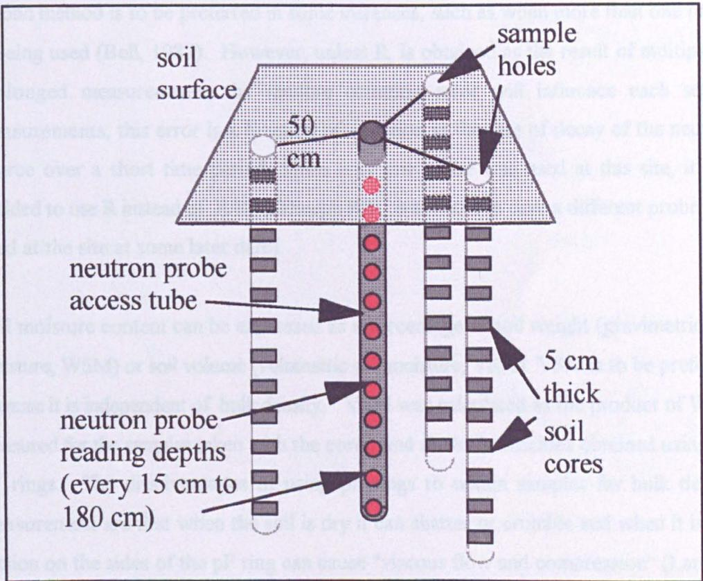
Figure 2.6 Soil sampling positions for neutron probe calibration.
