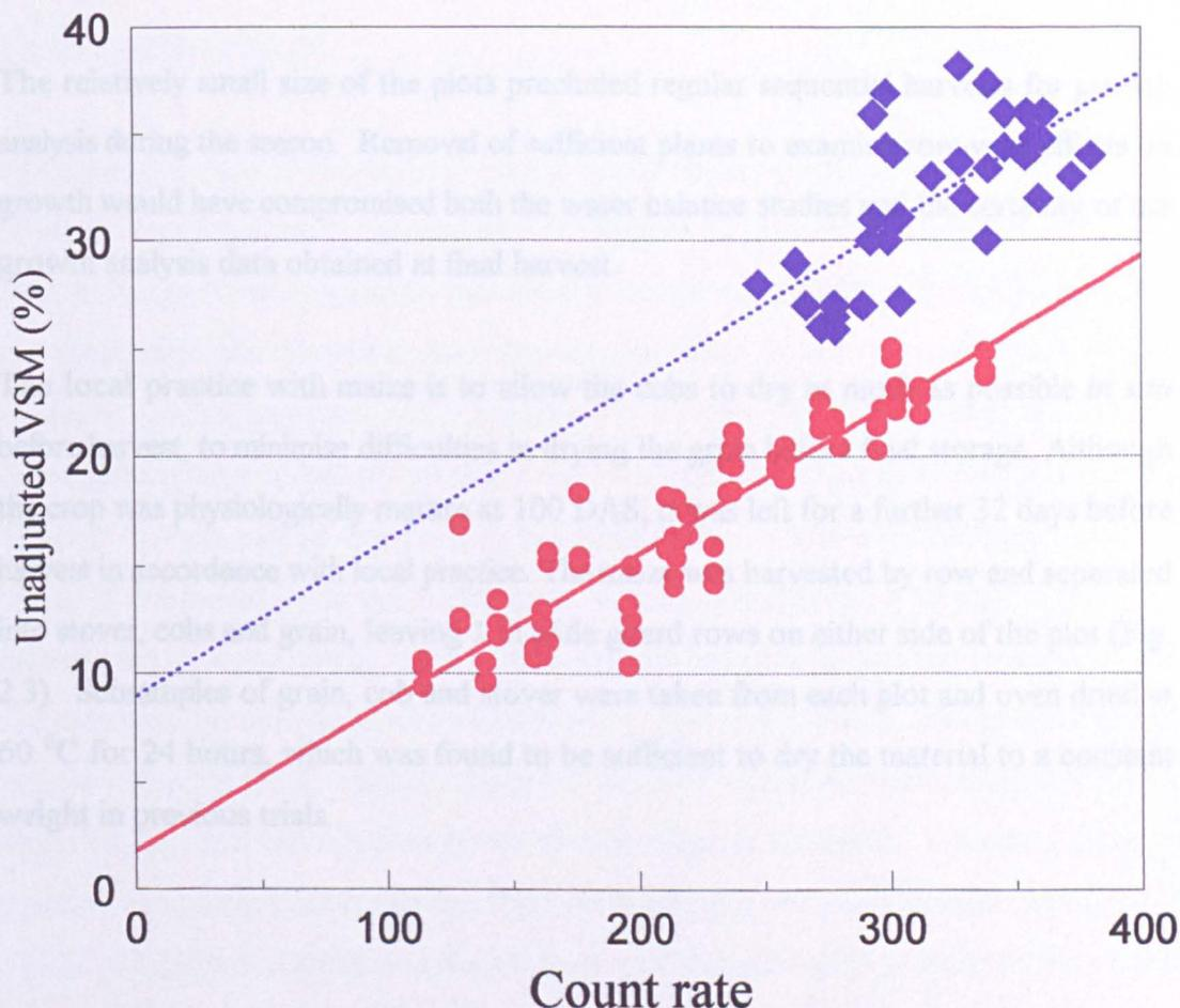
**Figure 2.8** Correlation between unadjusted volumetric soil moisture (VSM) and neutron probe count rate. Values are shown for core samples taken from dry soil ( $\bullet$ ,  $y = 0.069x + 1.84$ ,  $r^2 = 0.83$ ,  $n = 80$ ) or from pF ring samples taken from artificially wetted soil ( $\blacklozenge$ ,  $y = 0.072x + 8.95$ ,  $r^2 = 0.51$ ,  $n = 40$ ). Bulk density values for the wetted samples were used to calculate the volumetric soil moisture content.
