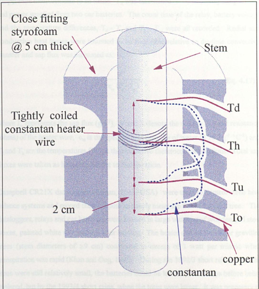
**Figure 4.18** Diagrammatic illustration of a heat balance gauge for measuring sap flux.  $T_d$ ,  $T_u$ ,  $T_h$  and  $T_o$  represent thermocouple positions. The styrofoam insulation and stem segments extending for 5 - 10 cm above and below the insulation were tightly wrapped in aluminium foil.
