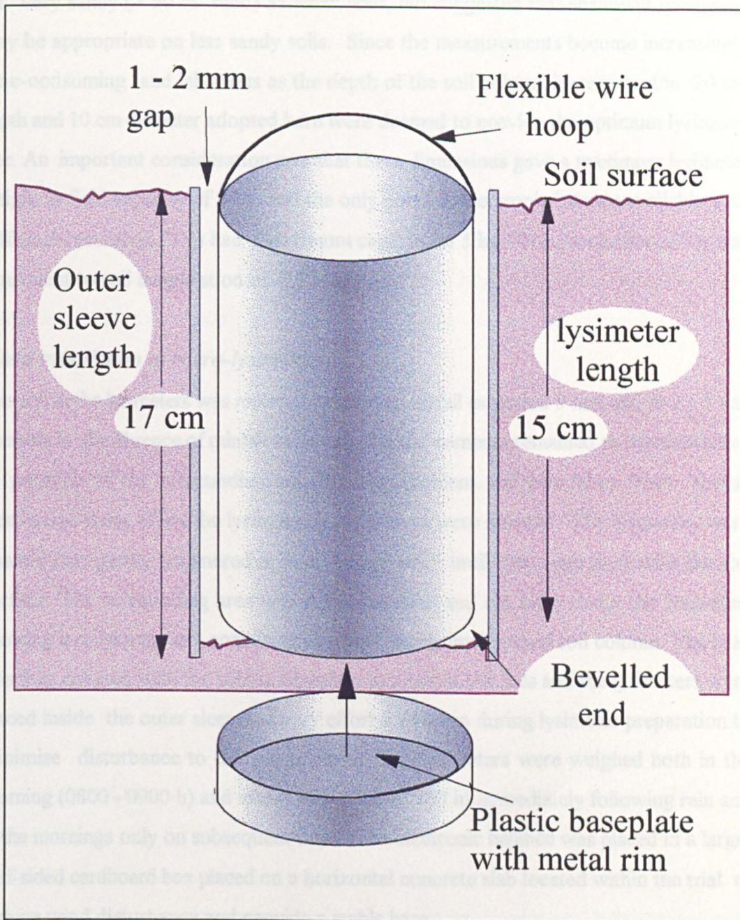
**Figure 4.22** Diagrammatic illustration of a micro-lysimeter used for measuring soil evaporation. The lysimeters and outer sleeves were constructed from 10 cm diameter PVC drainpipes. The micro-lysimeters, containing soil columns from locations representative of the outer sleeve sites, were located flush with the soil surface. The flexible wire hoops permitted easy extraction for weighing and were pushed to one side between measurements to minimise interference.
