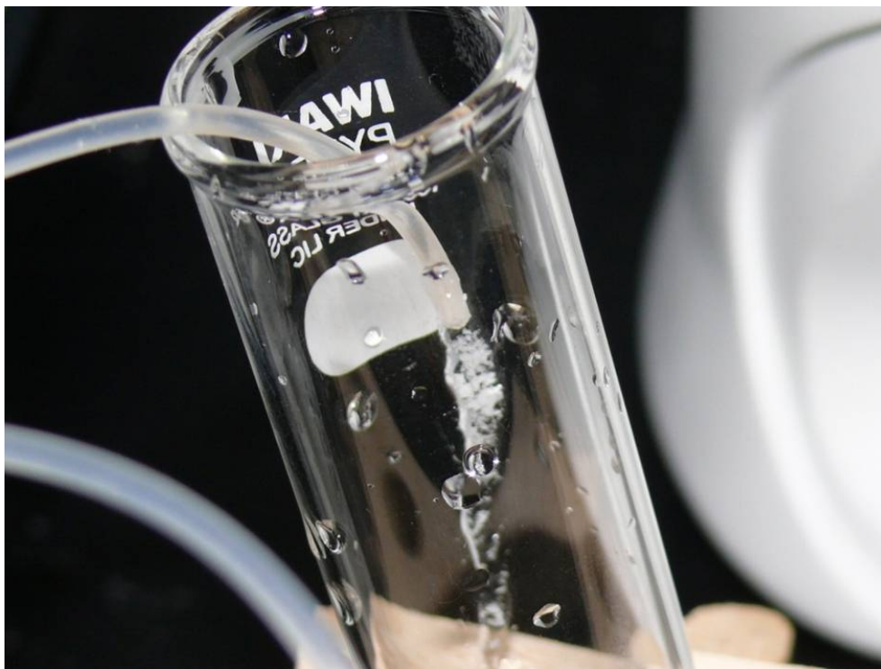
Figure 3.16: Crystal observation at the end of the output tube for 5.0% Saturated Paracetamol nucleation measurement experiments.
