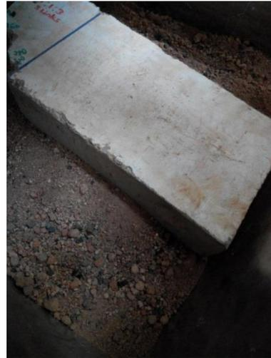
Figure 5.9: (a) The soil box that contains soil with a circular opening for entry of motion and (b) the concrete slab which acts as surcharge on the soil for the first 0.55 m after entry.
