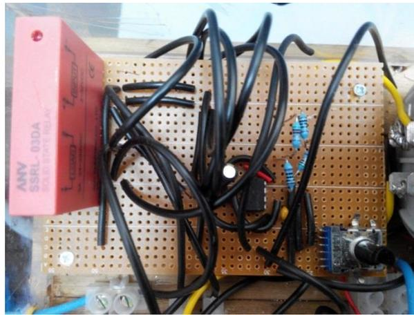
Figure 5.2: The circuit board LM555 the timer and potentiometer that manipulates the operating frequency of AC power supply.
