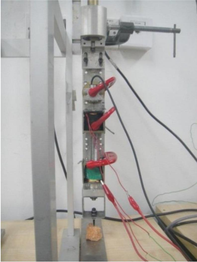
Figure 3.20: (a) Photograph of two degree-of-freedom electro-vibroimpact system.
