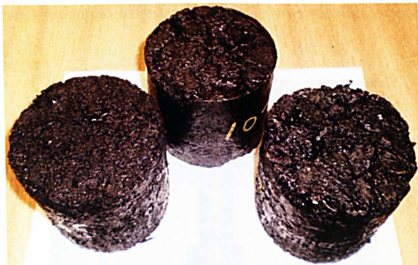
Figure 5.16 Specimen ready for compression testing
