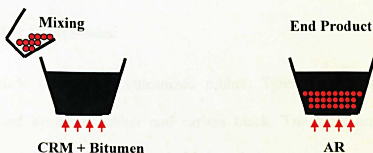
Figure 2.1 Wet process method
