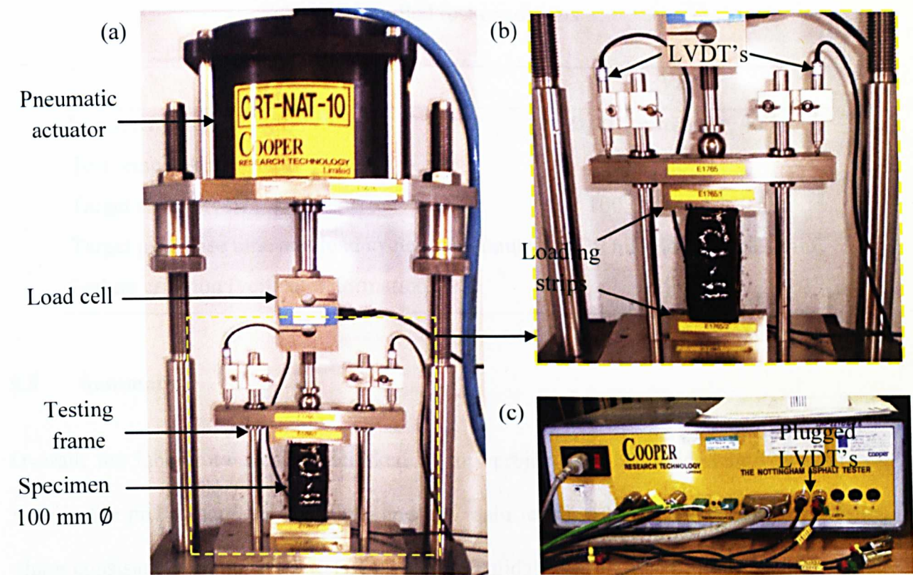
Figure 5.24 (a) Nottingham asphalt tester, (b) testing frame and (c) data logging equipment
