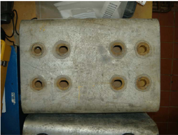
Figure 4.1 Shroud plate out of specification
