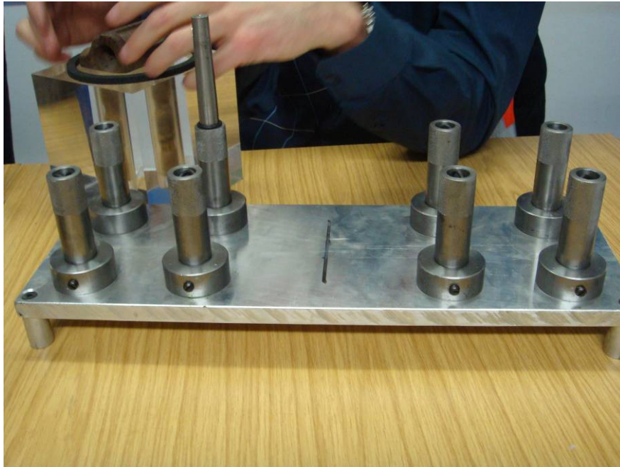
Figure 4.7 Cemex jig for insert placement
