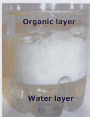
Fig. 5.30: Extraction of TBP-titania using post-modification process
