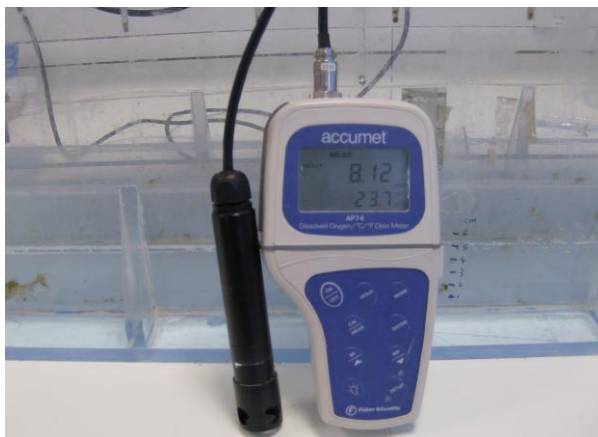
Figure III-11: Camera shot of Accumet waterproof AP74 DO meter along with the galvanic probe.
