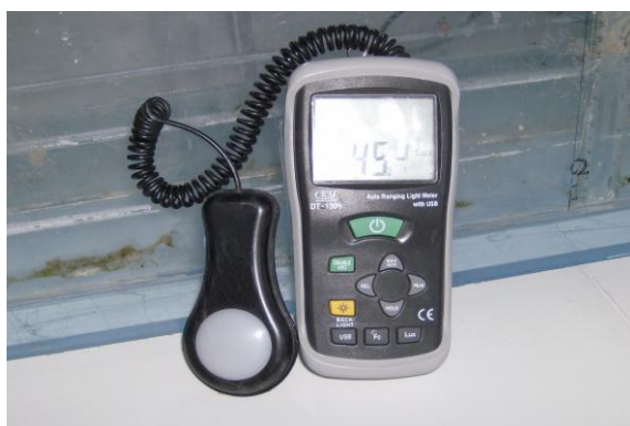
Figure III-12: Camera photo showing LX-319 Light meter and the connected light probe.
