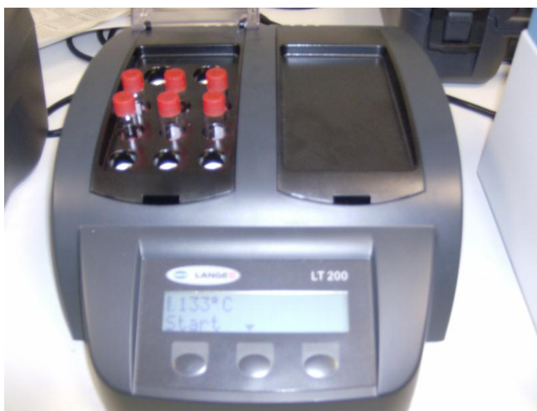
Figure III-14: Photograph showing COD reactor and COD cuvettes being kept for digestion.
