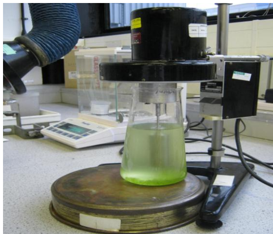
Figure III-16: Picture showing Brookfield Viscometer for viscosity measurement.
