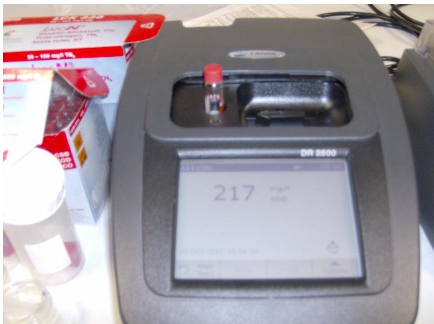
Figure III-13: Camera grab of Hach Lange DR 2800 Spectrophotometer reading the sample cuvette by automatic bar code identification.
