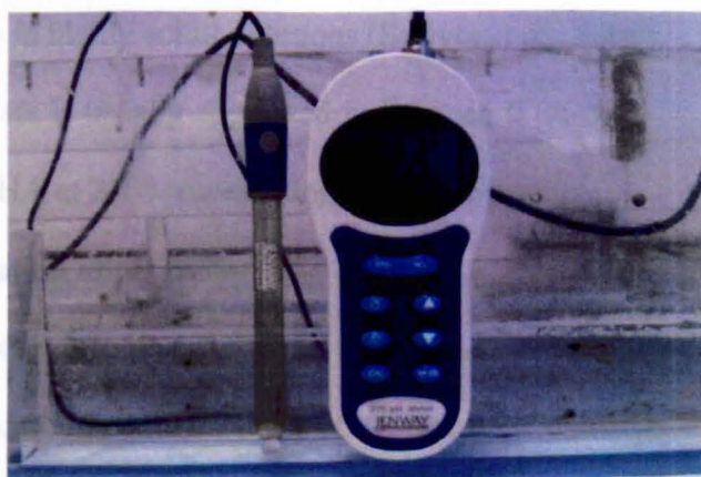
Figure III-10: Camera image of Jenway 370 pH meter with the attached probe.
