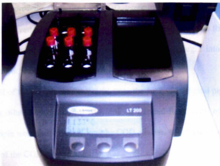
Figure III-14: Photograph showing COD reactor and COD cuvettes being kept for digestion.
