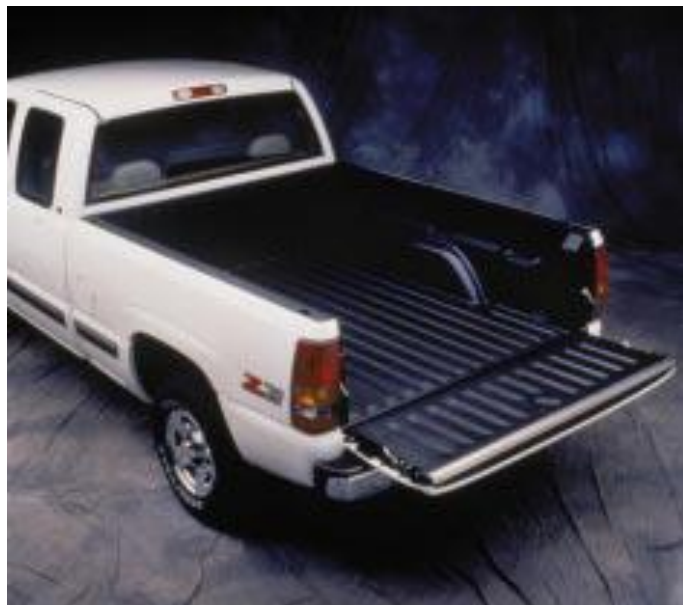
Figure 1-2 Composite truck bed installed in Chevrolet Silverado.
