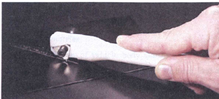
Fig. 3.13: Scribe tool recommended by Volvo Car Corporation [69]. Photo courtesy of VCC.
