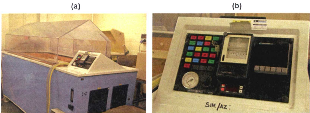
Fig.5.20: Corrosion cabinet (a) general view and (b) detail view of control panel. Photos courtesy of FMC.
