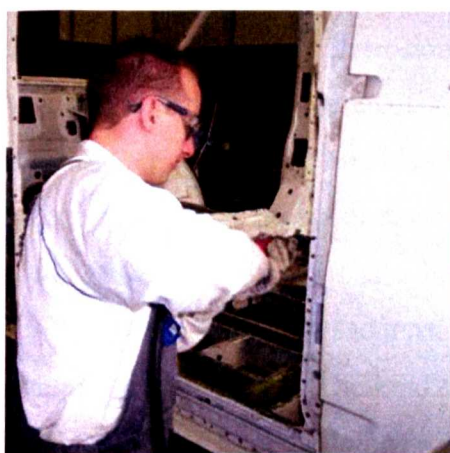
Fig. 3.4: Vehicle disassembly for tear-down analysis. Photo courtesy of Ford Motor Company Ltd. (FMC)
