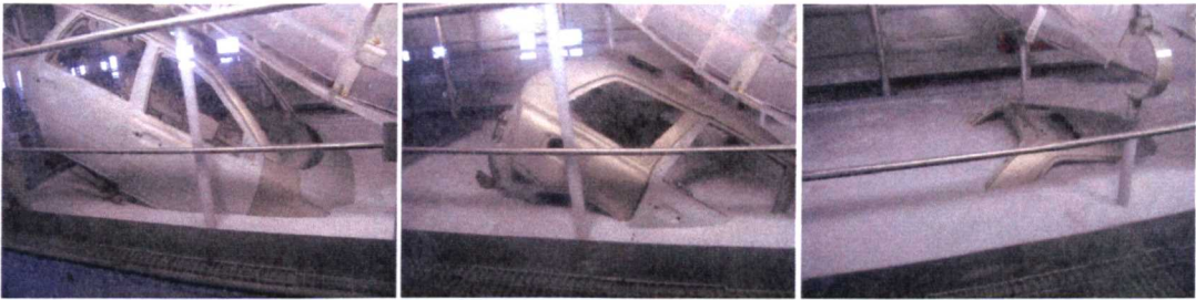
Fig. 5.4: Immersion of a vehicle body in the e-coat tank. Photos courtesy of VCC.
