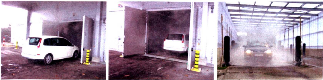
Fig. 3.10: Test vehicle ( left and centre ) entering the climate chamber and ( right ) driving through salt mist at Lommel Proving Ground. Photos courtesy of FMC.
