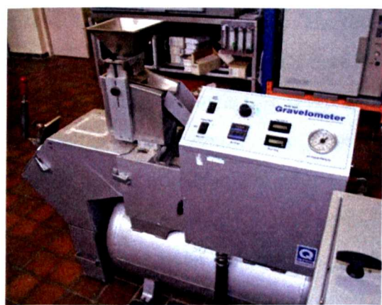
Fig. 3.12: Painted panel chipping apparatus. Photo courtesy of FMC.
