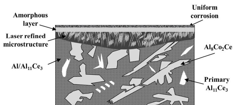
Figure 8-34 Schematic of the corrosion in the LSM-LAEB treated layer 1. Uniform corrosion occurred in the crack-free and compositionally homogeneous LSM-LAEB treated amorphous layer.
