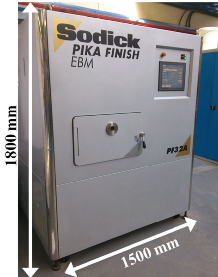
Figure 3-6 Large area electron beam machine used in this work (Sodick PF 32A).
