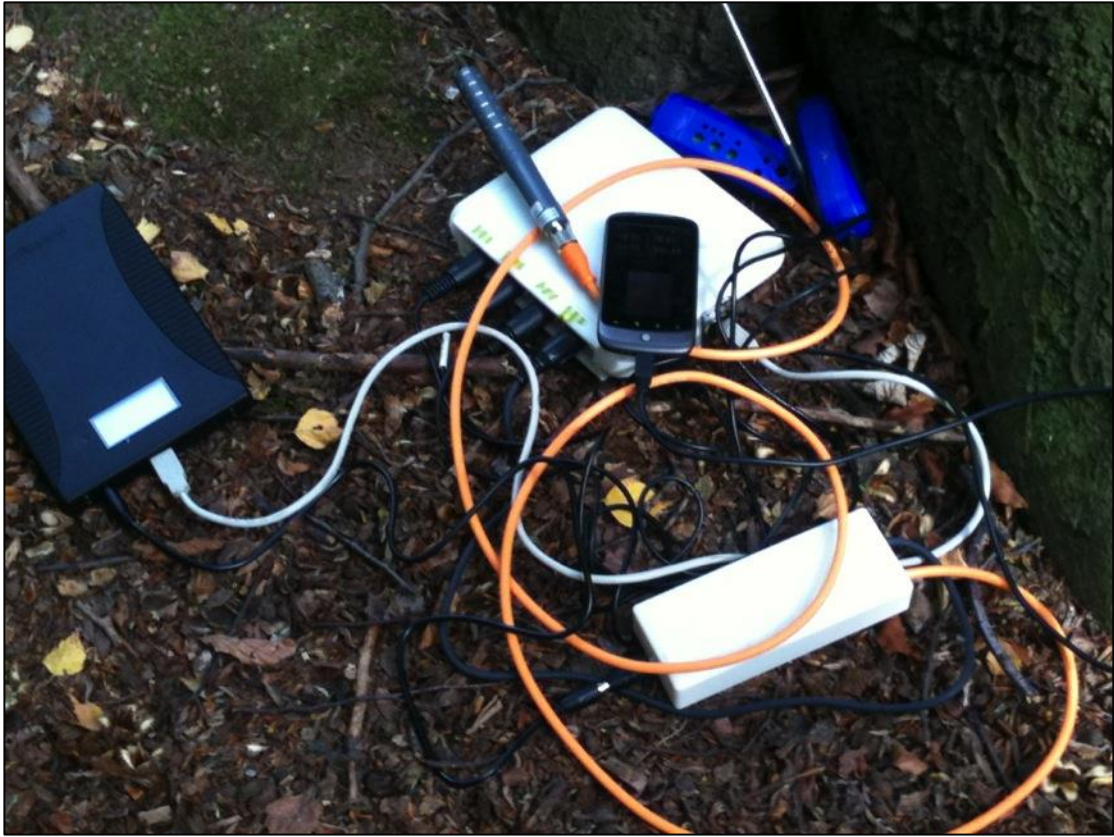
Fig.25 The new sensor kit including: C02 monitor, decibel sensor, humidity sensor, temperature sensor, Arduino hub, Android phone and Power Gorilla Battery
