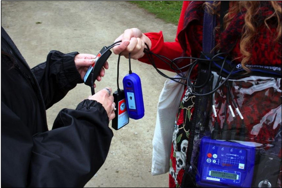
Fig.23 Old sensor kit including: Sciencescope hub, Nokia N95, temperature, humidity, atmospheric pressure and decibel sensors
