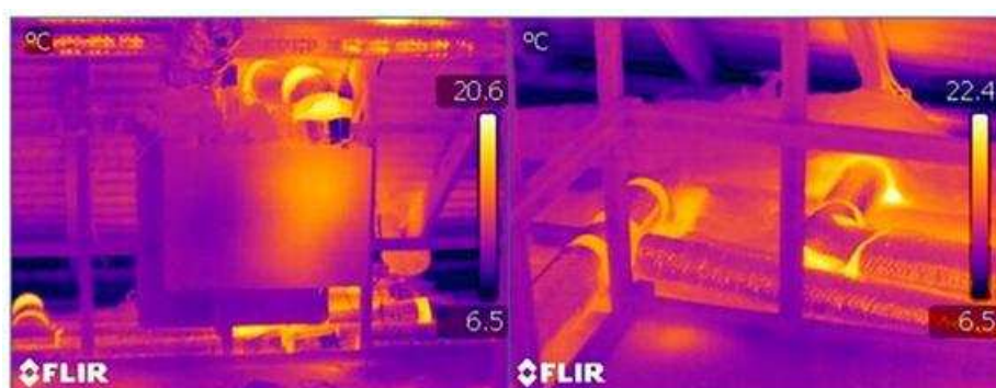
Figure 5-8 - Thermal Images of MVHR Control Unit & Duct Work
