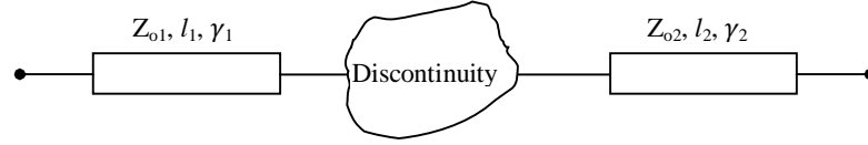
Fig. 2.15 Cascade representation of transmission line with discontinuity
