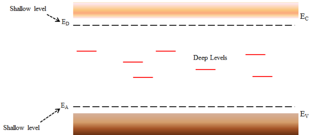
Figure 3.8: Schematic diagram of deep level impurities in semiconductors. E_D and E_A are shallow donor and shallow acceptor levels, respectively.
