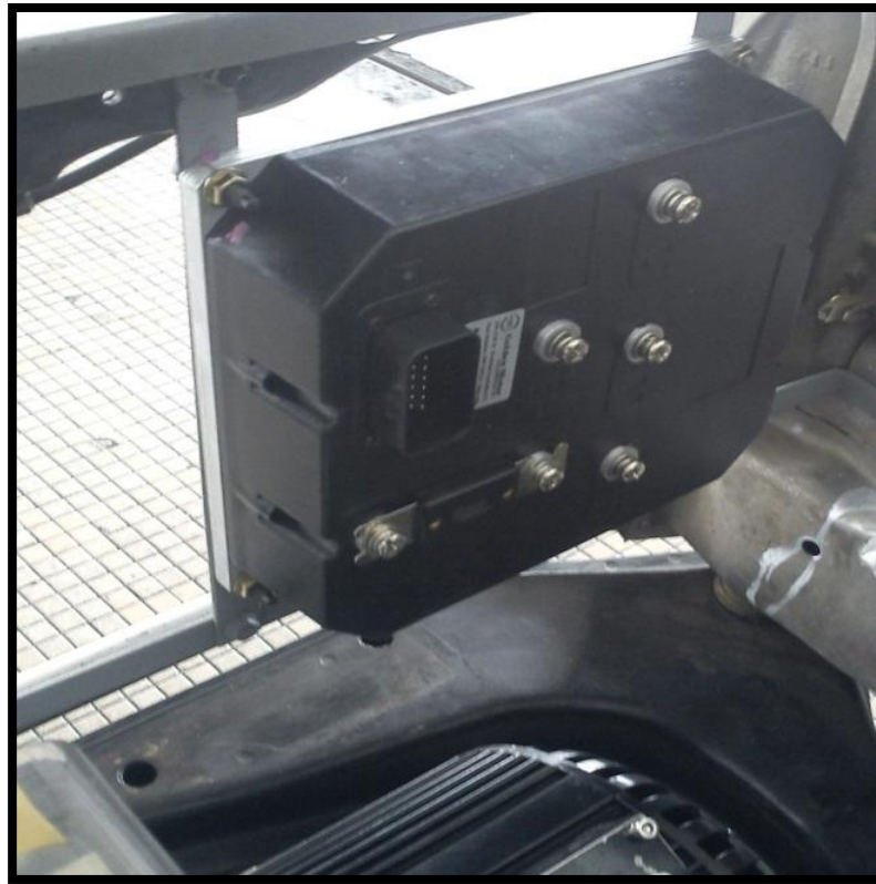
Fig 44: 500A Motor Controller successfully mounted in the same position as the radiator of a conventional vehicle
