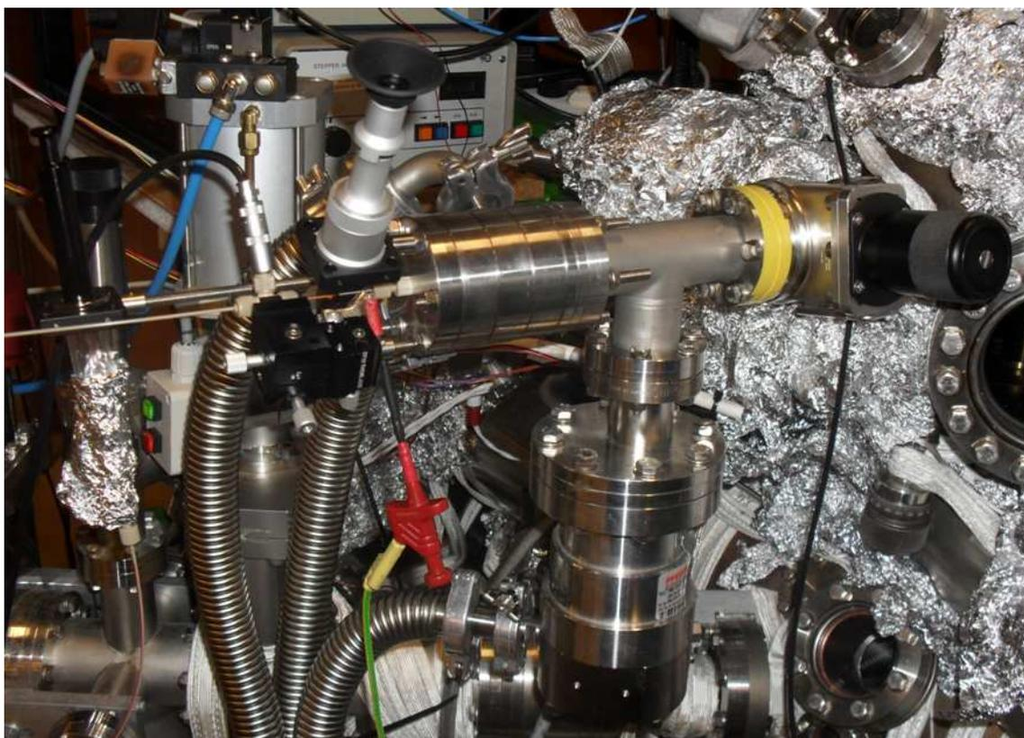
**Figure 5.5:** Photograph of a UHV electro spray system mounted onto the end chamber of beamline I311 at MAX-lab, Sweden. The syringe is covered in foil to help prevent the photodegradation of the molecules contained in the syringe. A microscope can be seen attached to the system to observe the electro spray plume, the red electrical connector has been used to ground the entrance capillary on the electro spray device.
