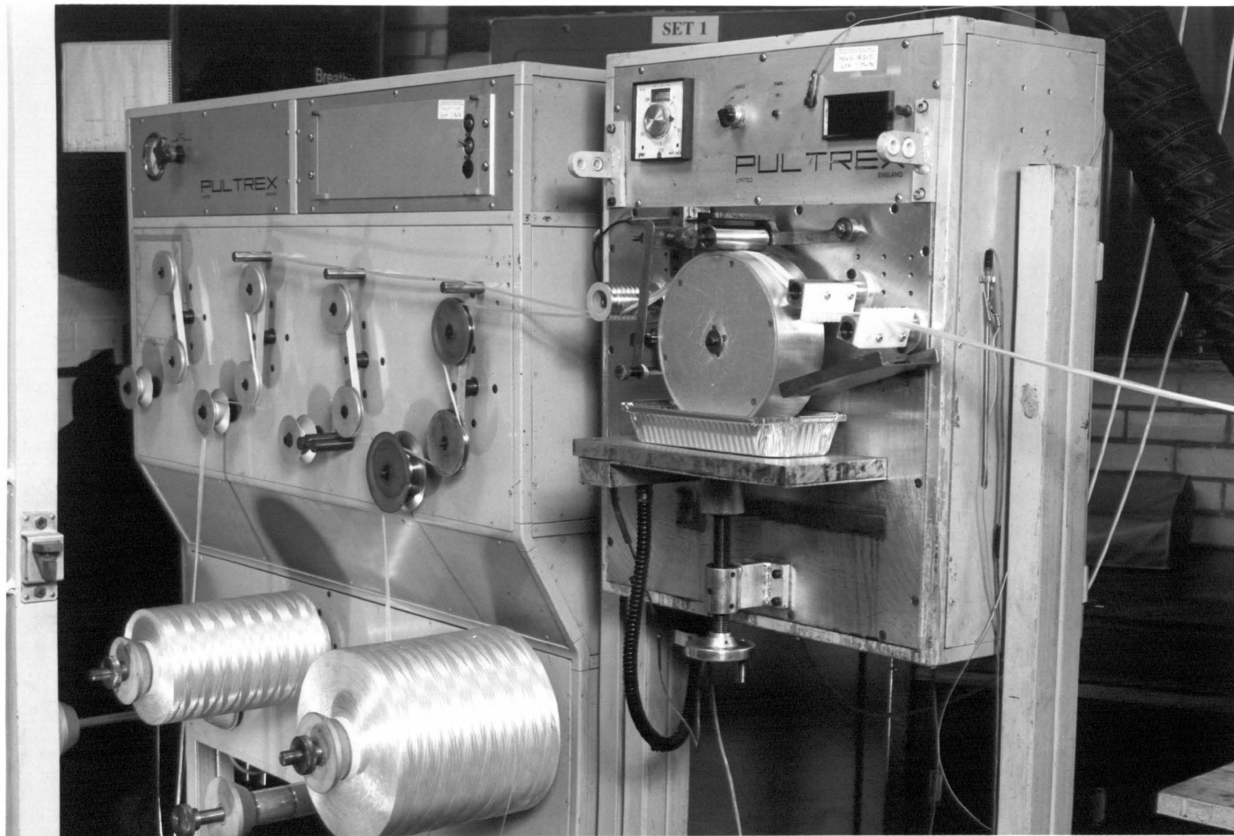
Figure 1-3: The Fibre Tension Controller and Resin Impregnation System
