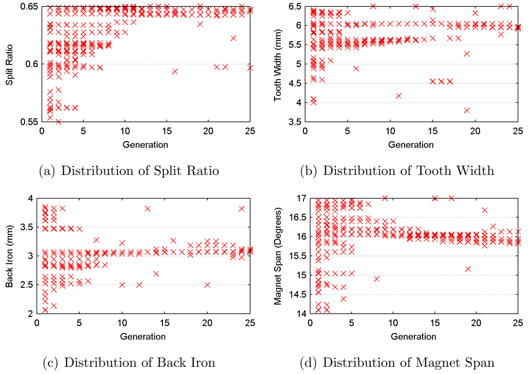
Figure 6.9: Stage one GA optimization of 24s20p topology
