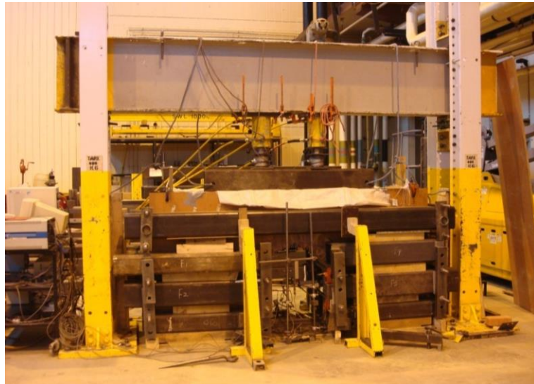
Figure 3.9 Loading system installation for uniform load
