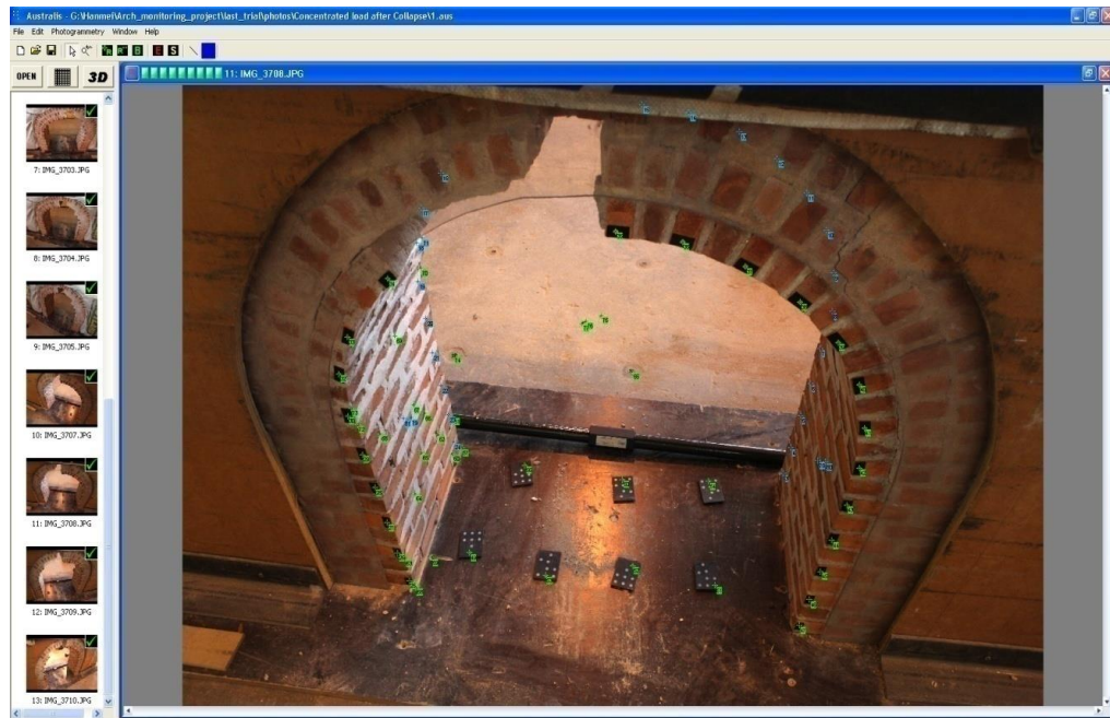
Figure 3.30 Dots and coded targets in green
