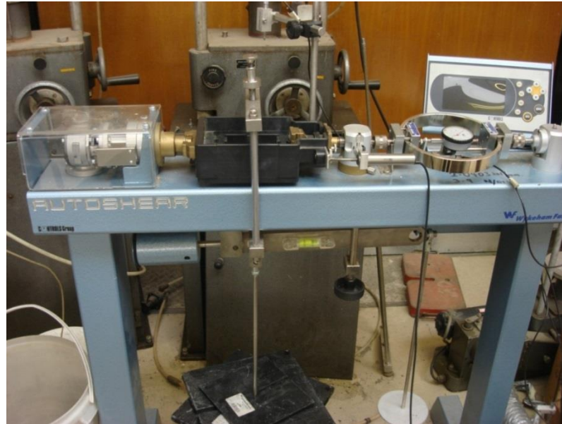
Figure 4.6 General view of shear box apparatus
