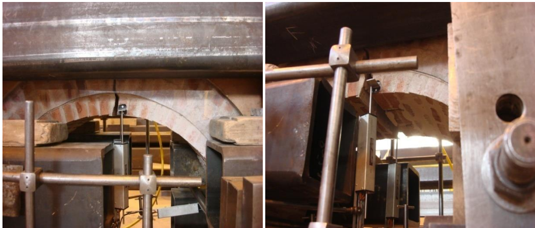
Figure 3.28 Structural hinge at tunnel crown along the width under concentrated load
