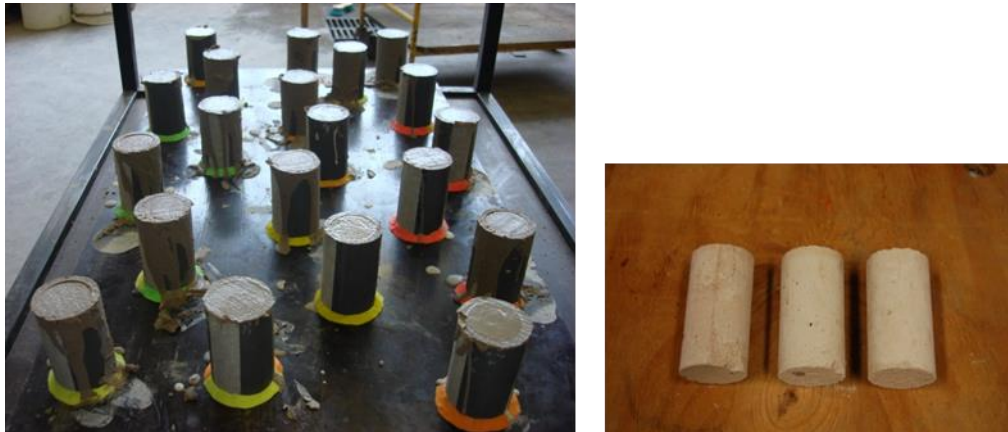
Figure 4.5 (a) PVC pipe sections for mortar sample preparation; (b) Mortar cylinder samples
