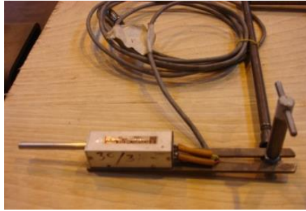
Figure 3.16 Potentiometer with 30 mm range
