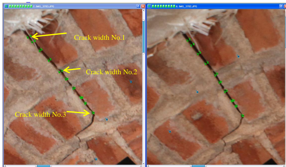
Figure 3.42 Non-targetted points of interest in coordinates along a major crack
