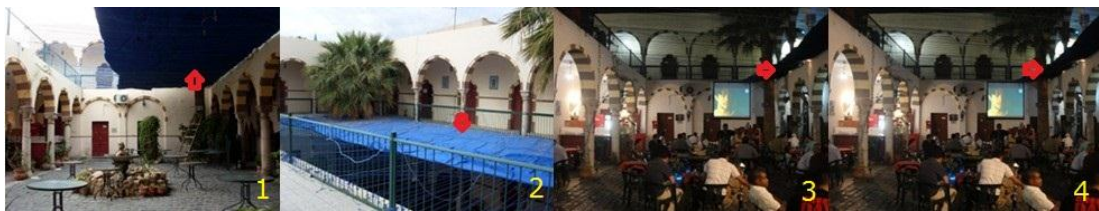
Figure 7-46: Photographs showing special structural adaptation measures (covering the courtyard during the winter season (1 &2) and removing the cover during the summer season (3 &4))
