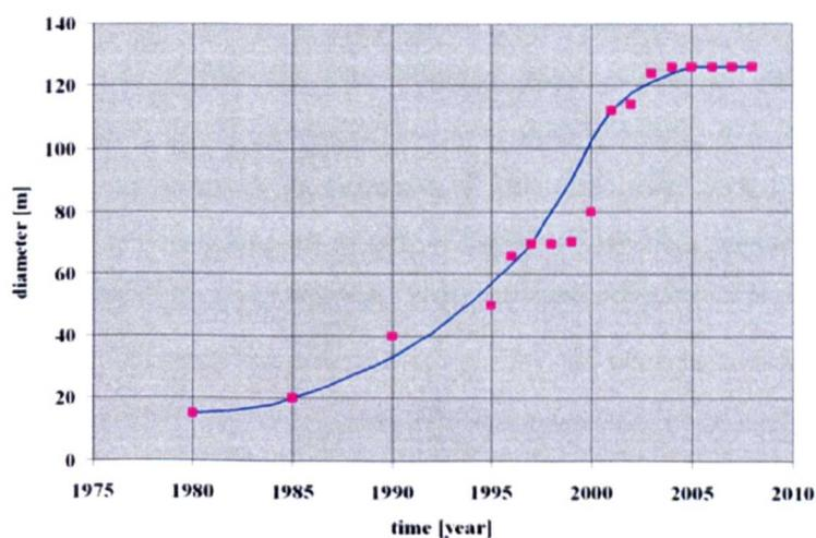
**Fig 1-2** The largest wind turbine diameters from 1980 to 2008 [7]
