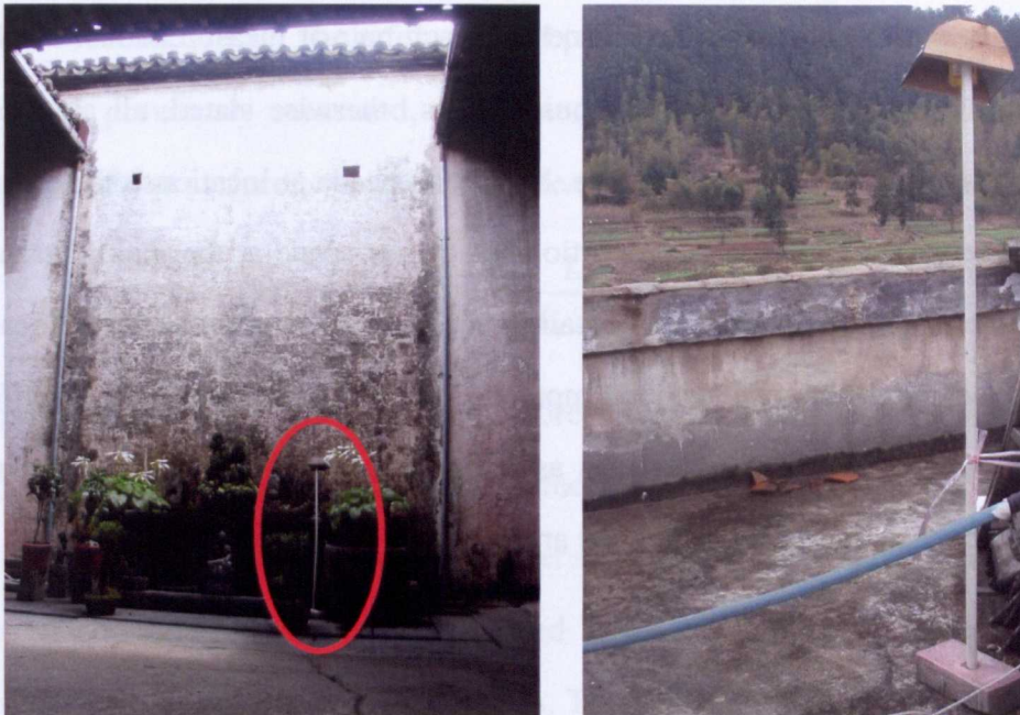
Figure 1. 2 Data loggers in skywells or on roof tops were protected by a curved cover
