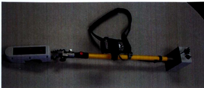
Figure 3.2 the Green Seeker Hand-Held model (505 Optical Sensor, NTech, Industries Inc )
