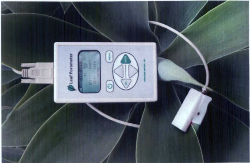
Figure 3.3 the Decagon SC-1 Leaf Porometer (Decagon Devices, Inc., Pullman, Washington)
