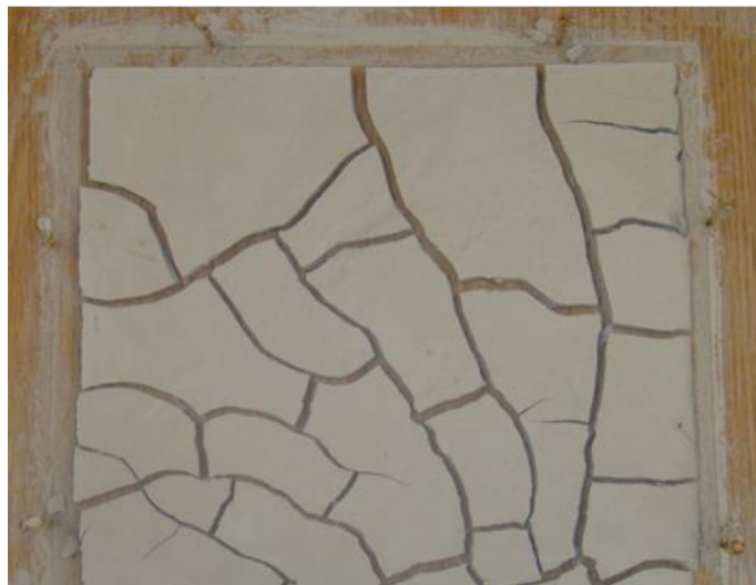
Figure 5-28 A panel made of 90% clay and 10% MPCM, showing enormous cracks on the surface of the in panel.
