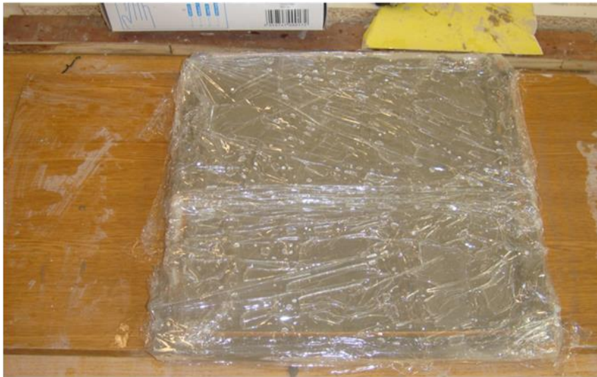
Cling film used for curing to minimize and avoid cracks.
