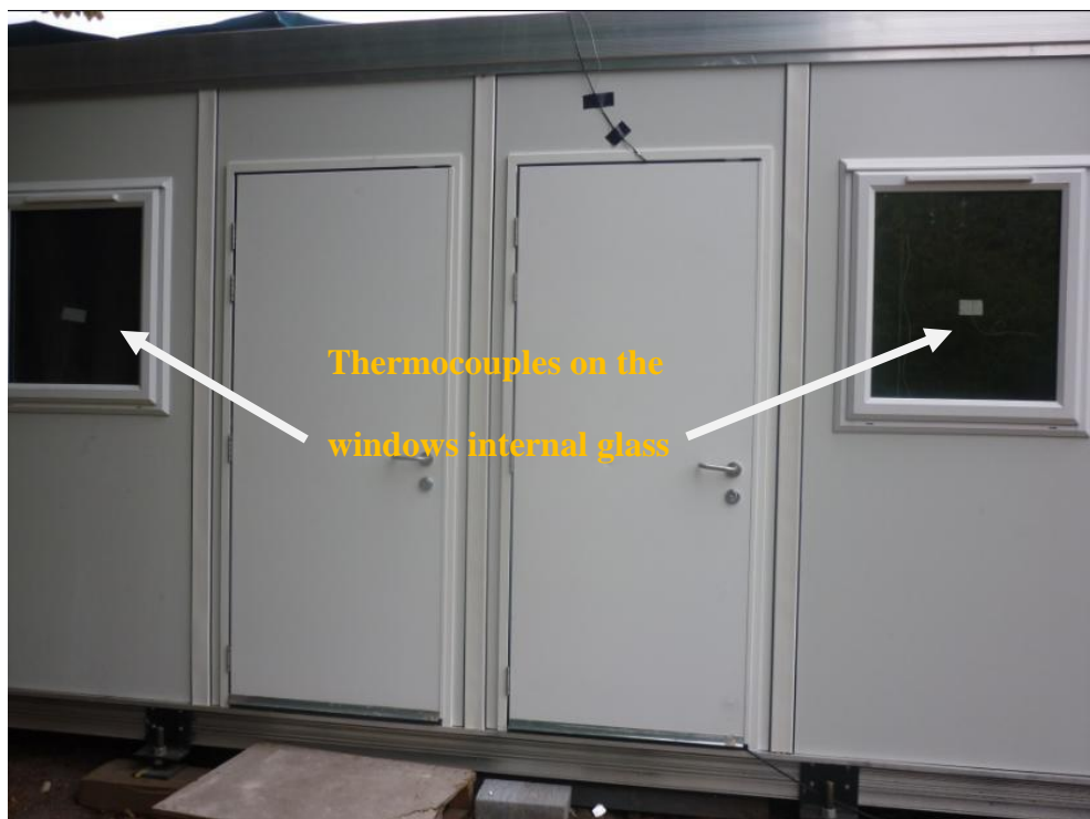
Figure 7-30 the position of the thermocouple on both windows.
