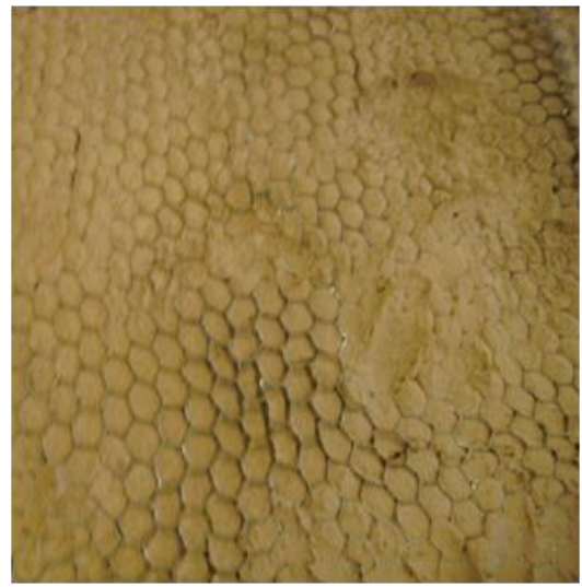
Figure 7-16 Place the mixture on the panel Figure 7-17 Honeycomb placed through the mixture.
