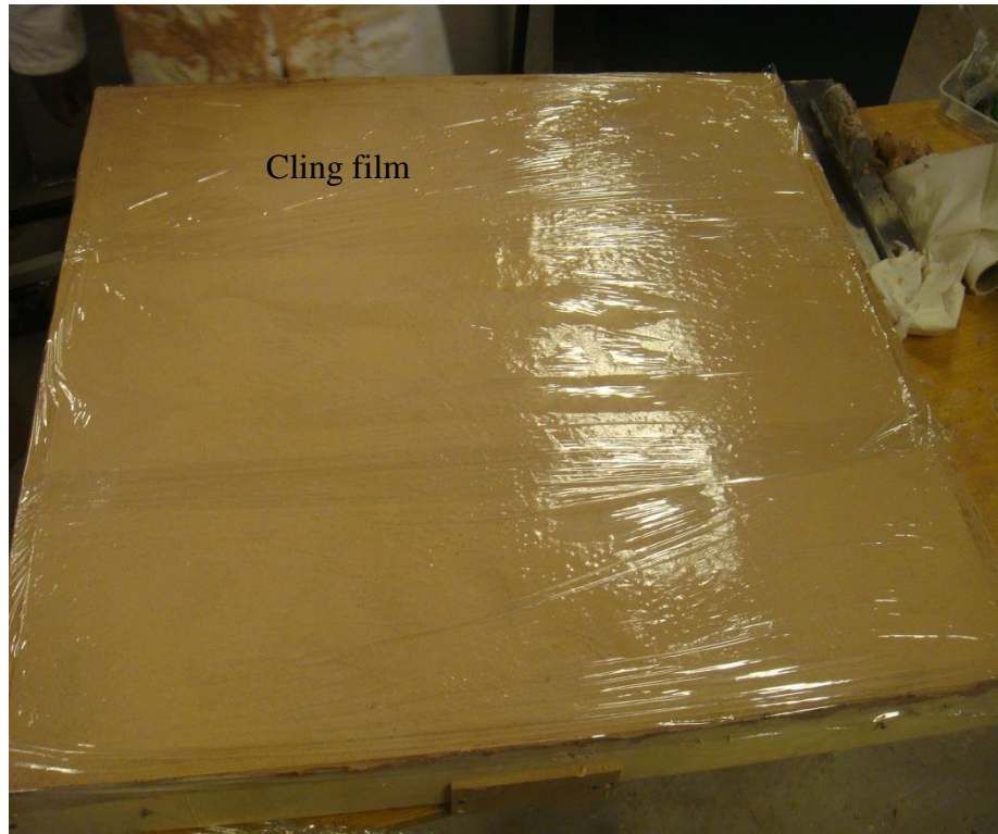
Figure 7-18 Curing process with a cling film.
