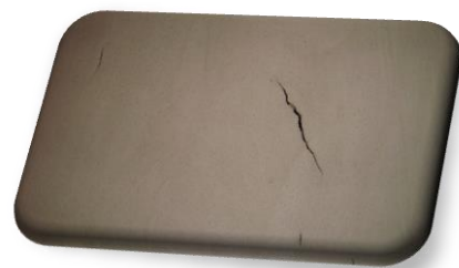
Figure 5-27 100% clay panel showing Crack appear on the surface of the panel.
