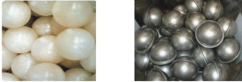
Figure 3-5 Plastic and steel PCM container (Kenisarin and Mahkamov, 2007)
