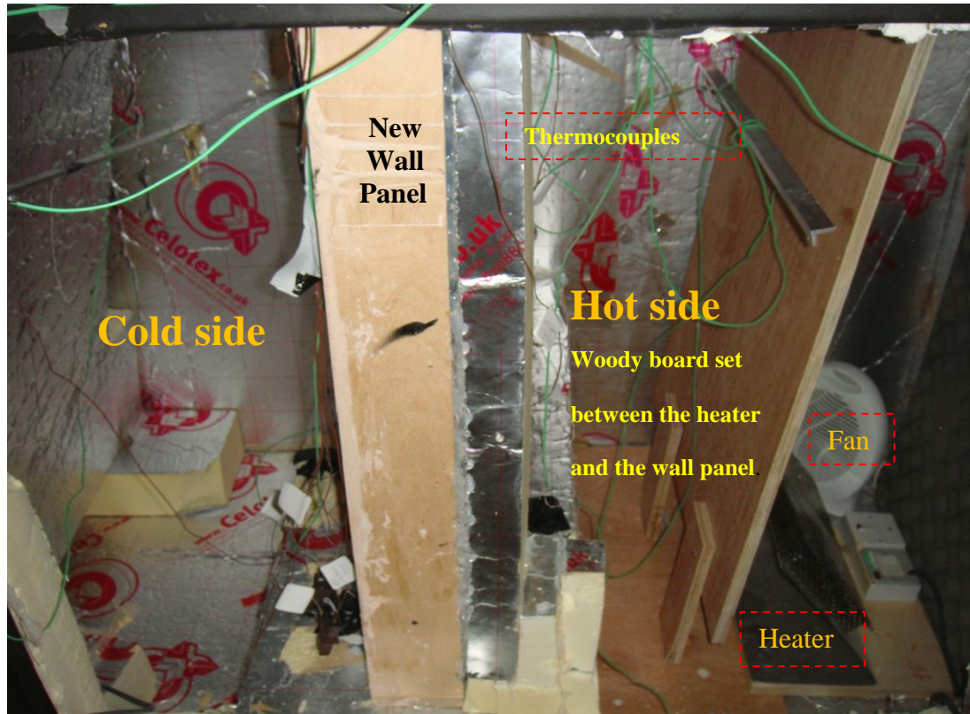
Figure 7-14 The hot side and the cold side of the test box, heater and the fan.
