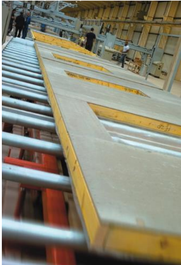
Figure 2-8 Timber frame wall panel manufactured in the Space4 factory (Lovell, 2012)
