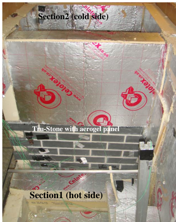
Figure 4-5 Tru-Stone with aerogel panel in the middle of the test room.
