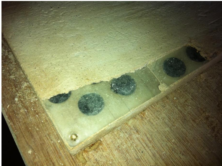
Figure 8-1 Adding encapsulate the PCM into gypsum panel.
