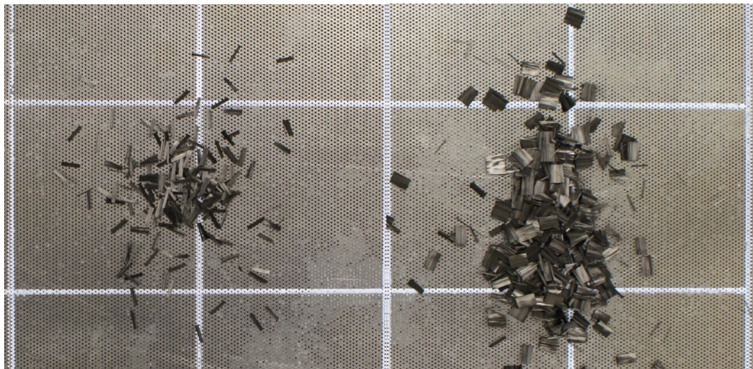
Figure 55. Increased fragmentation observed with 24k tows (right) compared with 3k tows (left). Note that the masses are different as each deposition used 1.8 m of fibre to achieve the same number of chopped tows.
