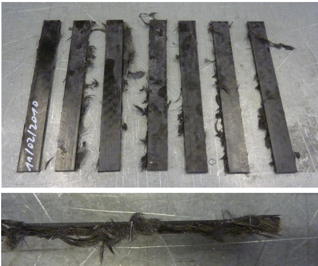
Figure 110. Dry RFPM trial specimens. Although top and bottom surfaces of some plaques looked satisfactory a dry region through the centre resulted in specimens that could not be tested. Plaques were cut by a water cooled diamond saw cutter. As specimens were cut dry fibre clung to the blade resulting in filamentisation of any dry fibre tows.
