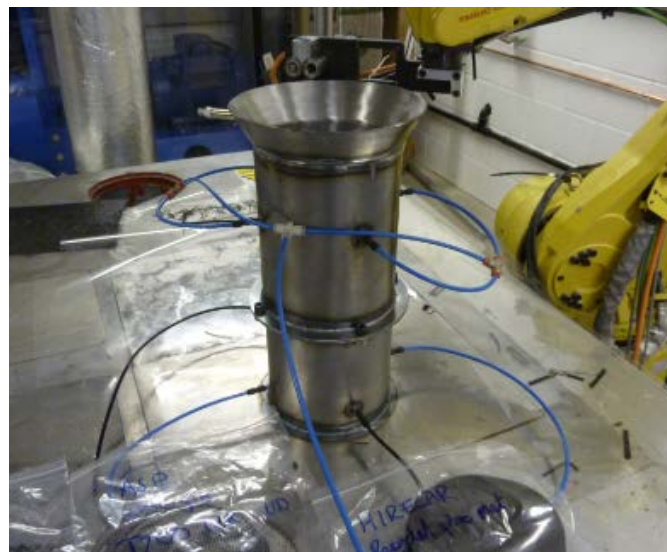
Figure 5-2: Experimental setup with the test duct positioned in place of the perforated screen.
