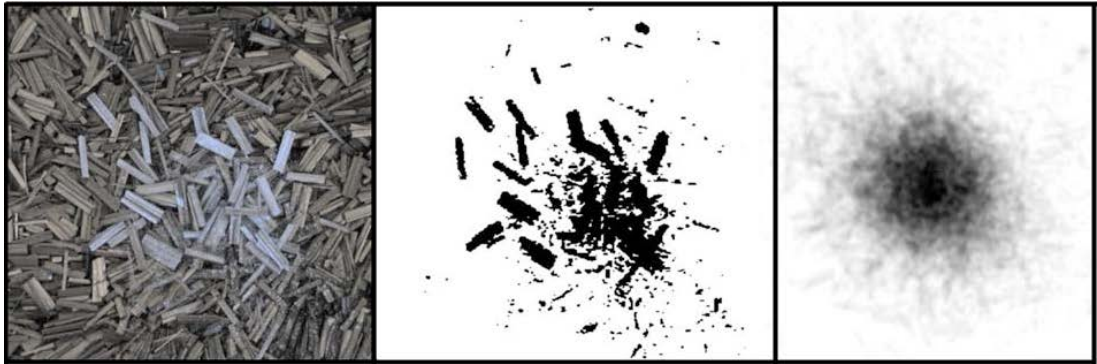
Figure 2-4: (Left) Picture of a discrete fibre deposition (coloured fibres) onto a surface already covered fibres. (Centre) A Digital image of the deposited fibres and (Right) the representative mass distribution after 20 sparse depositions. Images taken from [111].
