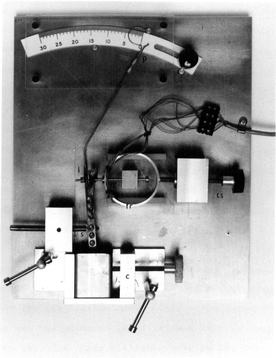
using an integrated circuit differential amplifier, which was calibrated together with the force ring transducer to allow a direct digital reading of the load applied in kilograms.
