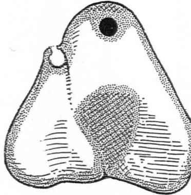
FIGURE 3.12 : Diagram of tibial plateau to show site of insertion of rod. The hatching marks the line of attachment of the synovium. The rod is inserted anteriorly into the tibial tuberosity, outside the joint cavity.
