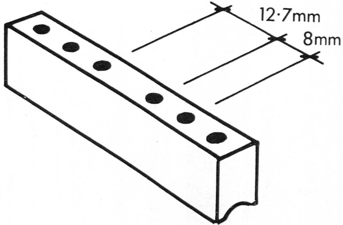
FIGURE 3.4 : Diagram of the drill guide. (Reproduced, with permission, from Ashurst et al 1982).
