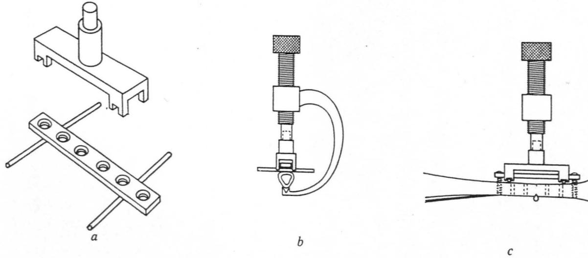
FIGURE 3.7 : The fracture device and C-clamp. (a) The fracture device and position of the rods in relation to the plate. (b) Transverse view of the device, rods and C-clamp on the bone. (c) Lateral view of the position of the instruments on the bone before fracture. (Reproduced, with permission, from Ashurst et al 1982).
