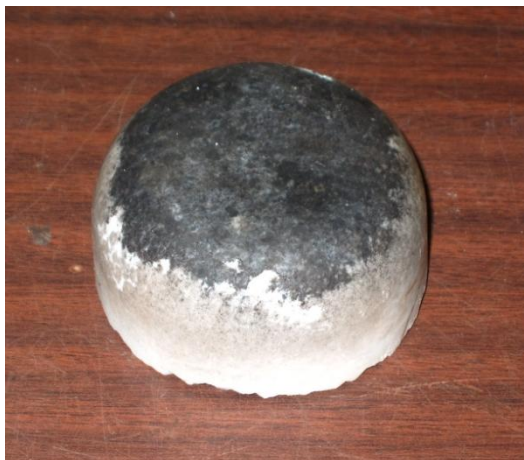
Figure 7.4: Solidified electrolyte removed from the reactor after carbon electro-deposition experiments in a \text{Li}_2\text{CO}_3\text{-Na}_2\text{CO}_3\text{-K}_2\text{CO}_3 electrolyte at a temperature of 702 °C. Note that the electrolyte has been placed upside-down so that the black material at the bottom of the electrolyte can be seen.
