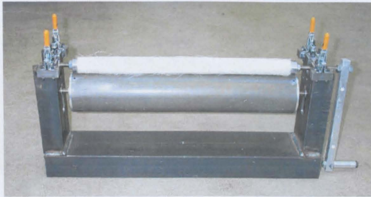
Figure 3-5 – Hand operated preforming rig for 38.1mm diameter tubes
