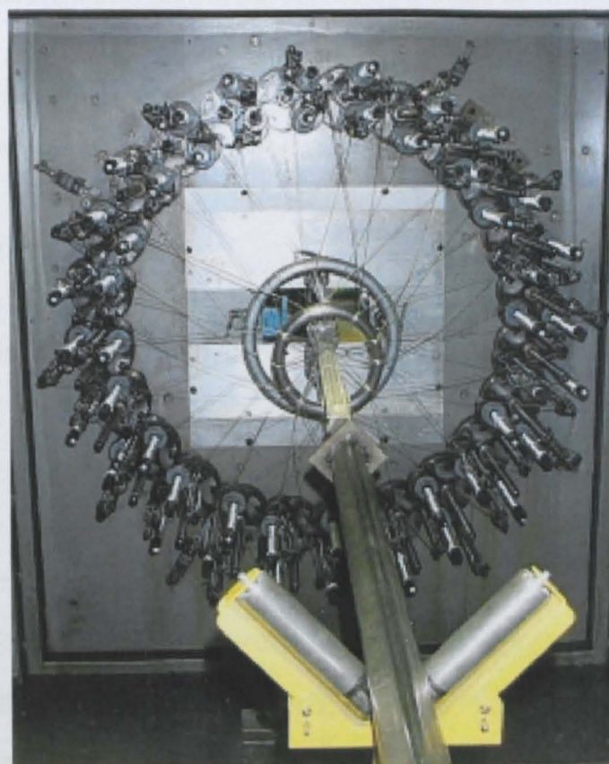
Figure 3-6 – The braiding of the 38.1mm diameter small braided tubes
