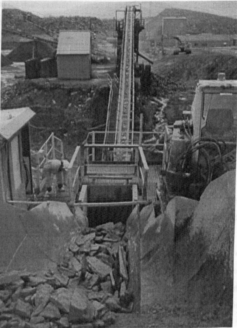
Figure 2.6 Processing of slate waste as Type 1 and 2 sub-base material.
