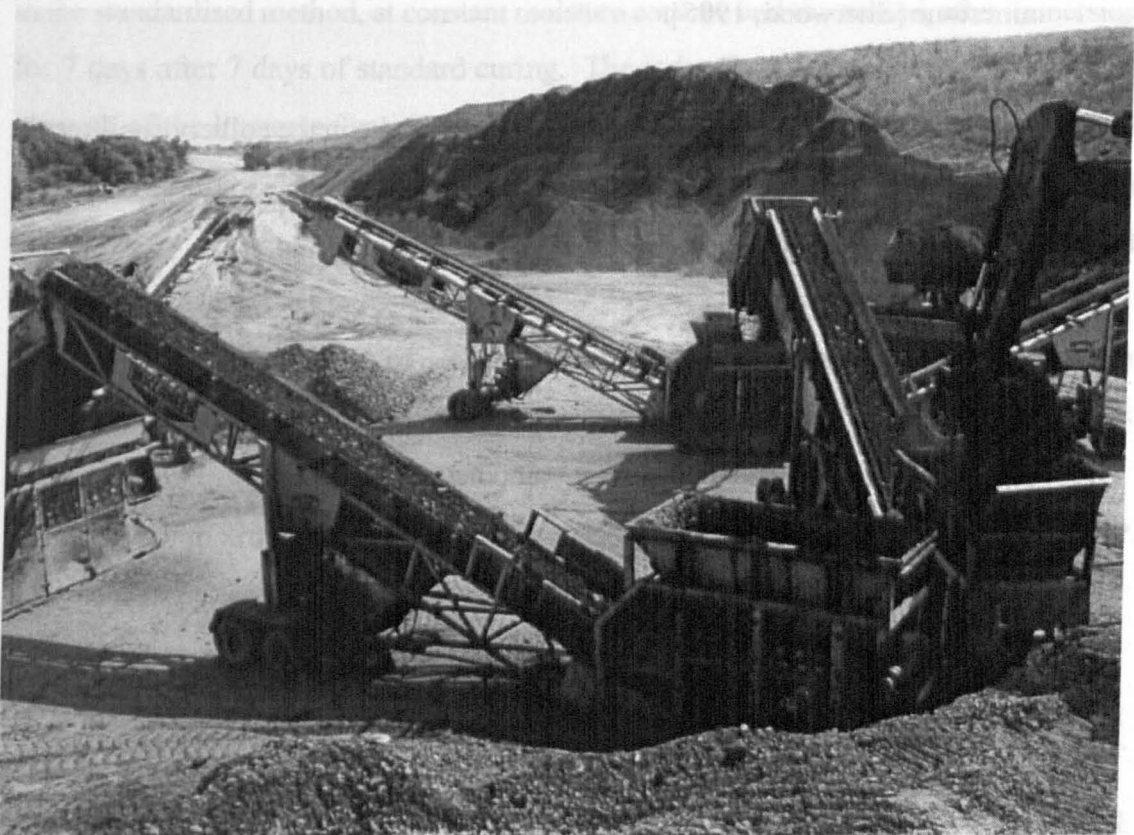
Figure 2.2 Processing of minestone at Gascoigne Wood Mine, Yorkshire.
