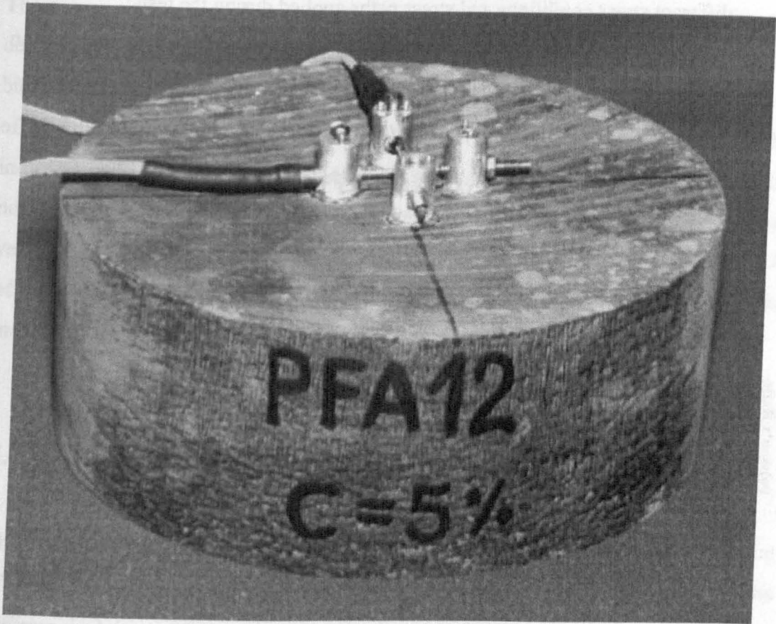
Figure 7.6 Measuring system used for determining Poisson's ratio.
