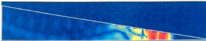
Figure 7.4.20: Pulse propagation in wing structure using fraction boundary placement model
