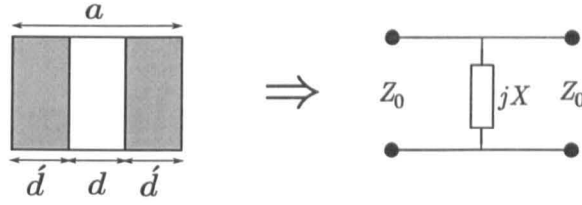
Figure 5.2.11: Waveguide slot aperture and its equivalent circuit [50]
