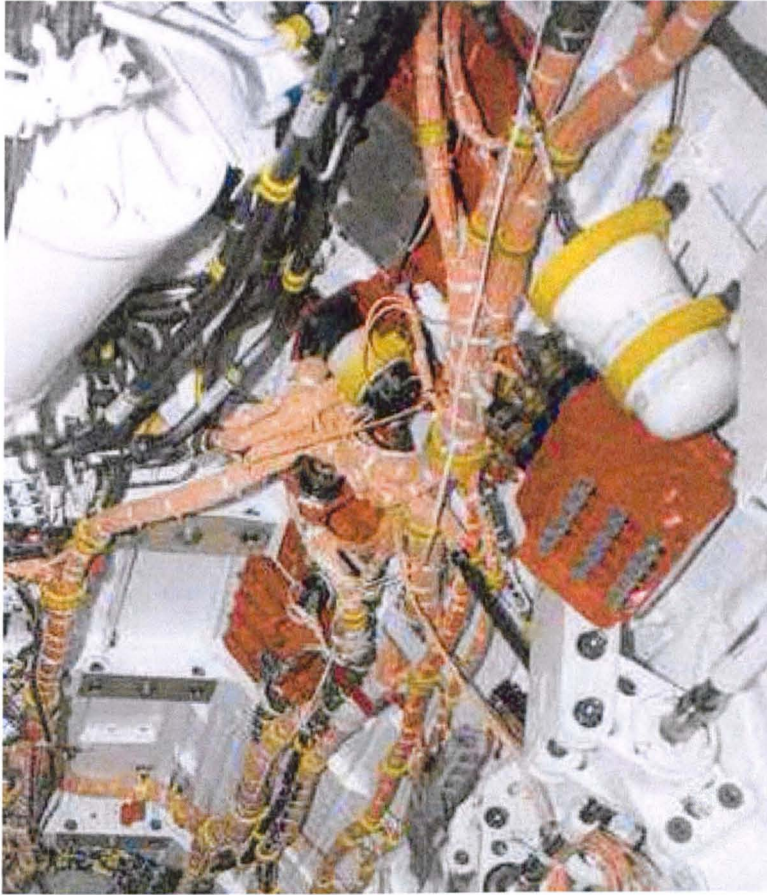
Figure 1.1.1: Equipment bay and wiring within the JSF [2]
