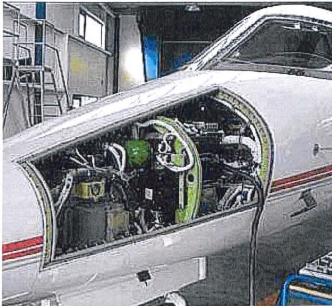
Figure 1.2.3: Equipment bay within a small civilian aircraft
