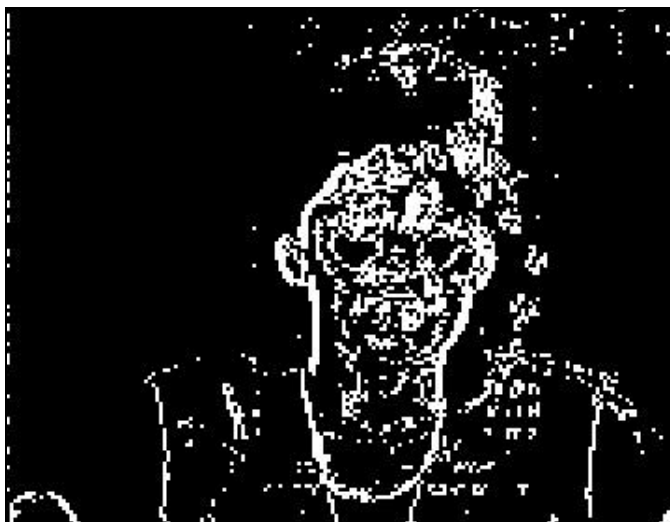
Figure 6.6.3: Location of motion vector origins, Miss America frame 032, DQ=8 , QCIF resolution
