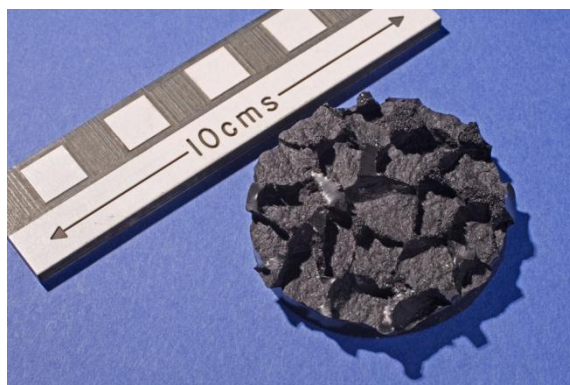
Figure 4.4 Replicated aggregate specimen
