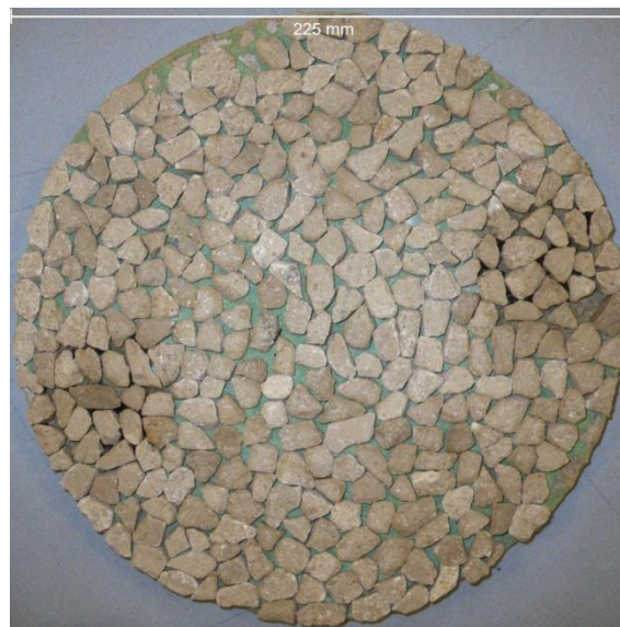
Figure 5.5 Limestone aggregate test specimen
