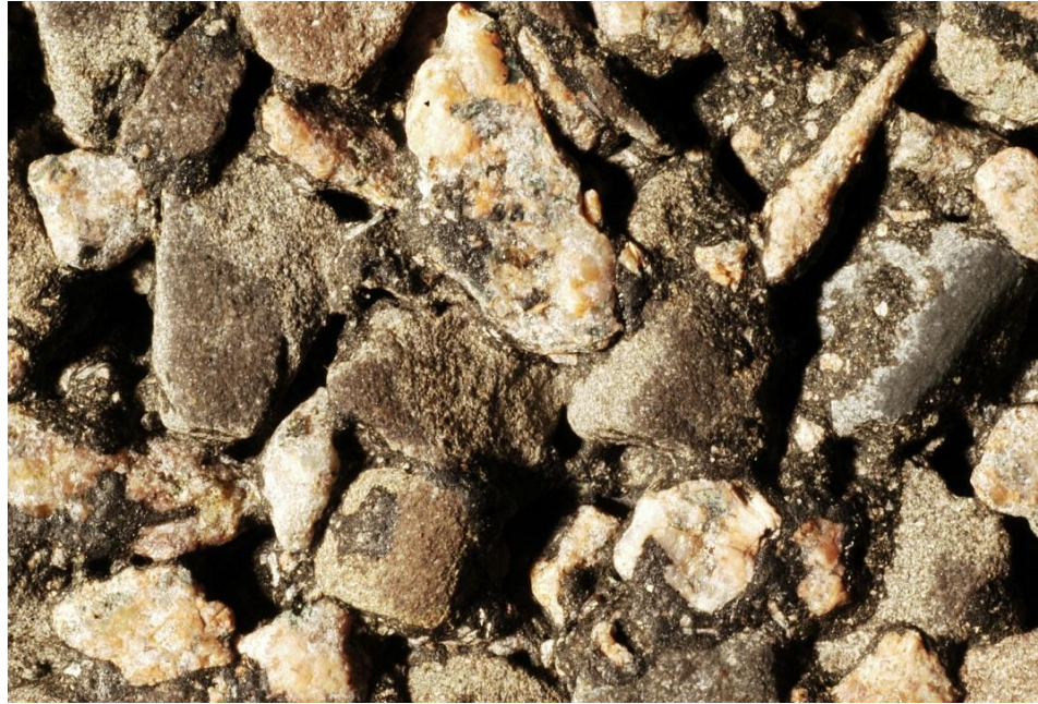
Figure 3.5 Photograph of polished asphalt specimen
