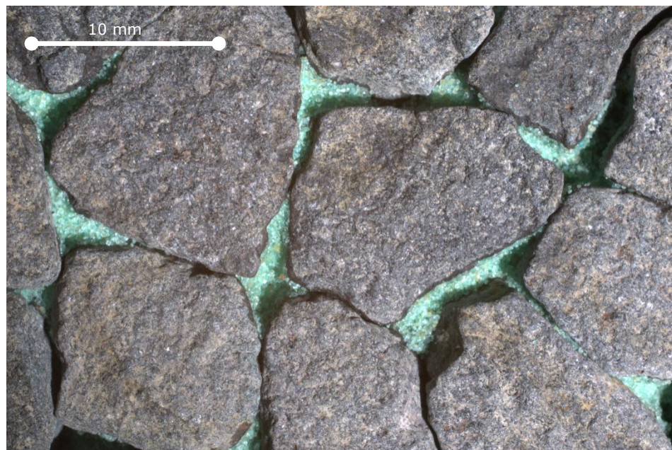
Figure 4.2 Dolerite aggregate specimen prepared for polishing
