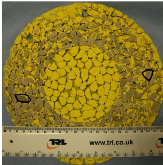
Figure 5.19 Limestone test specimen after painting and polishing
