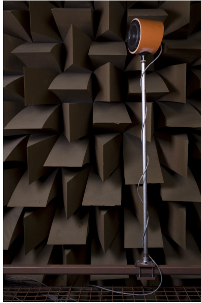
Figure 2.12: One of 48 custom built speakers inside the AEC. The speakers are placed along the horizontal in 10^\circ increments. Full description and schematic of the speakers is provided in [64]
